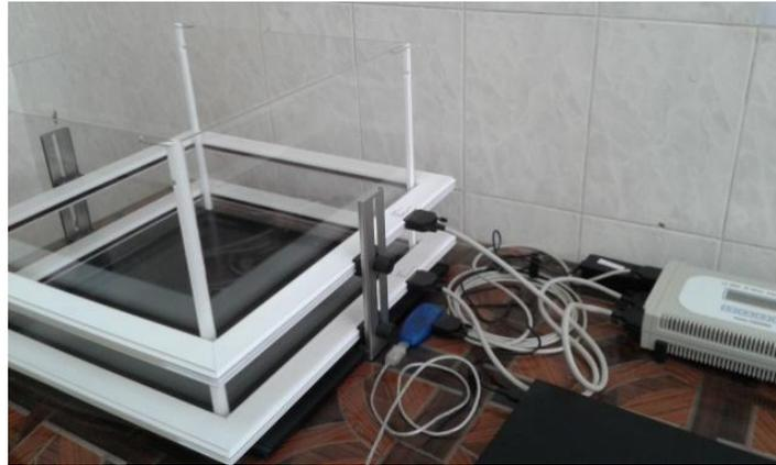
**Fig. 1:** Infrared LE8811 Actimeter (Panlab) apparatus for motor activity tracking in rats. Lower frame is used to track horizontal movements, while the upper frame tracks vertical movements (rearing).
