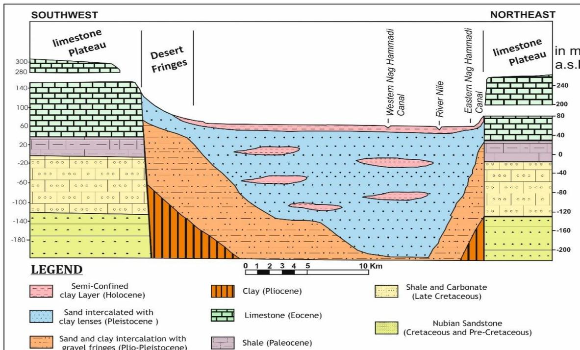
Fig. 3. The hydrogeologic cross section at Girga district, modified after [21].
