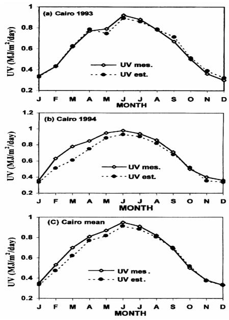
Fig. (3): Comparison between measured and estimated values of ultraviolet solar radiation at Cairo site for (a) 1993, (b) 1994 and (c) the mean.
