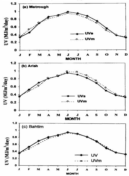
Fig. (5): Comparison between estimated values of ultraviolet solar radiation at (a) Matrough, (b) Arish and (c) Bahtim sites and the measured values Cairo site.
