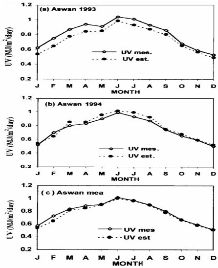
Fig. (4): Comparison between measured and estimated values of ultraviolet solar radiation at Aswan site for (a) 1993, (b) 1994 and (c) the mean.
