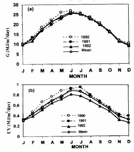
Fig. (1): Measurements date during the period (1990-1992) at Cairo station for (a) Global solar radiation (G) and (b) Ultraviolet solar radiation (UV).
