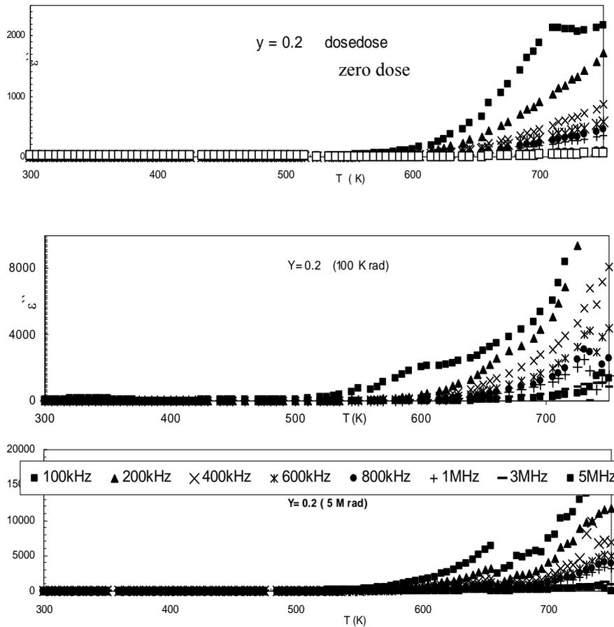
**Fig. (5):** Variation of dielectric loss with the absolute temperature at different Frequencies for irradiated and un irradiated Ce doped Co – Zn ferrite.
