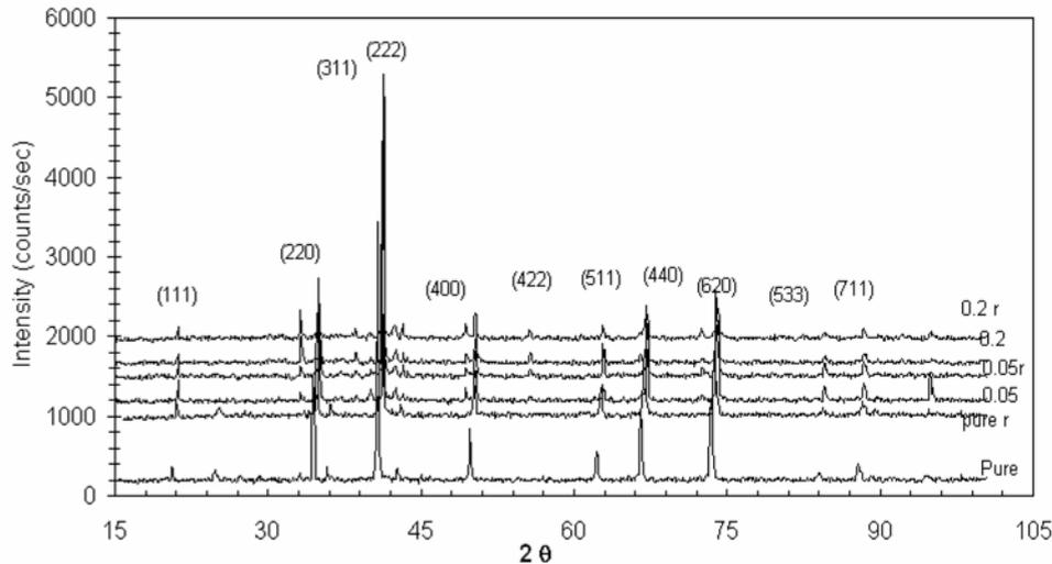
**Fig.(1):** X-ray diffractograms for radiated and unirradiated  $\text{Co}_{0.5}\text{Zn}_{0.5}\text{Ce}_y\text{Fe}_{2-y}\text{O}_4$
