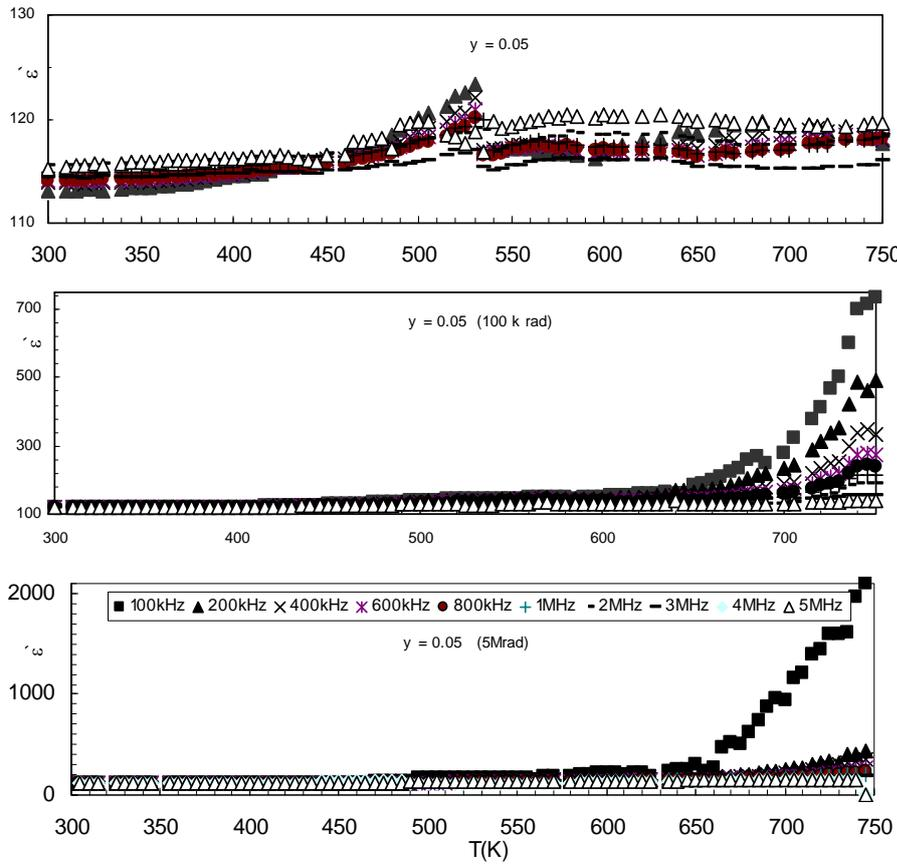
**Fig.(3):** Variation of the real part of the dielectric constant with the absolute temperature at different frequencies for irradiated and un-irradiated ferrite samples.
