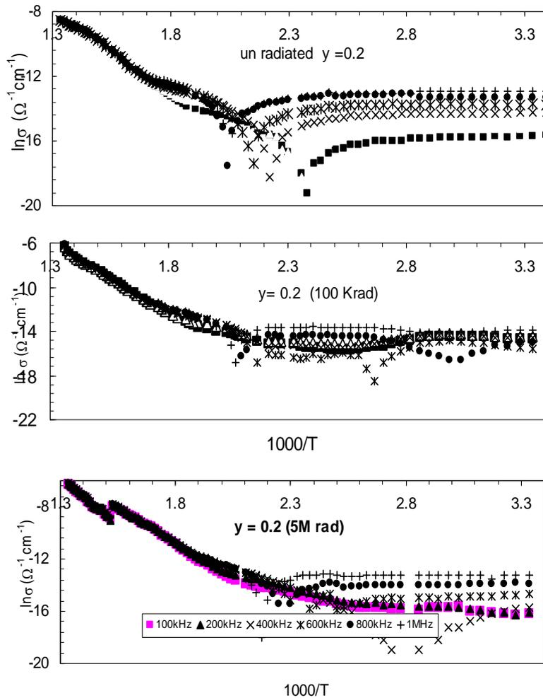
**Fig.(6):** Variation of ac conductivity ( $\ln \sigma$ ) with the reciprocal of absolute temperature ( $1000/T$ ) for irradiated and un irradiated Co- Zn ferrite samples.
