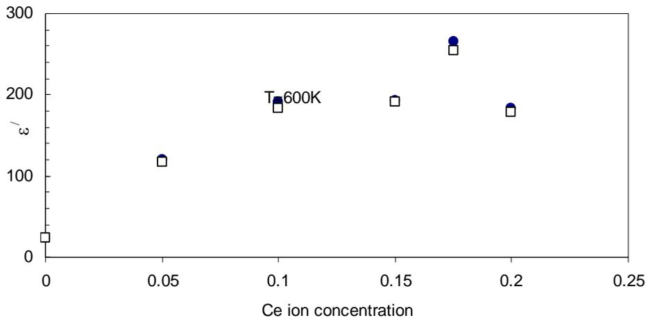
**Fig. (4):** Effect of Ce ion concentration on the real part of the dielectric constant
