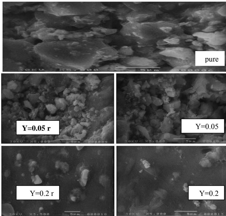
**Fig.(2):** The scanning electron micrographs for un irradiated and irradiated samples.
