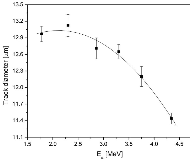
**Fig. (2):** The variations of the track diameter as a function of  $\alpha$ -particle energies at constant flux.
