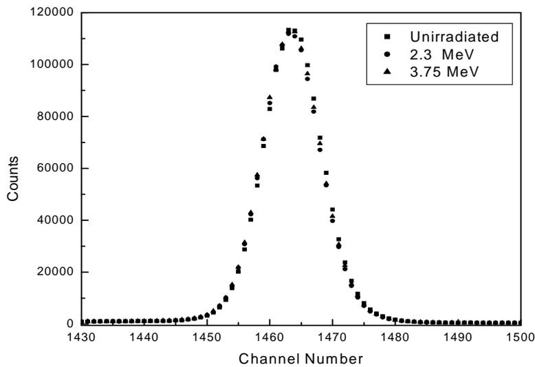
**Fig. (3):** The line shape spectra of the unirradiated sample and those irradiated with  $\alpha$ -particle energies of 2.3 and 3.75 MeV at constant flux.
