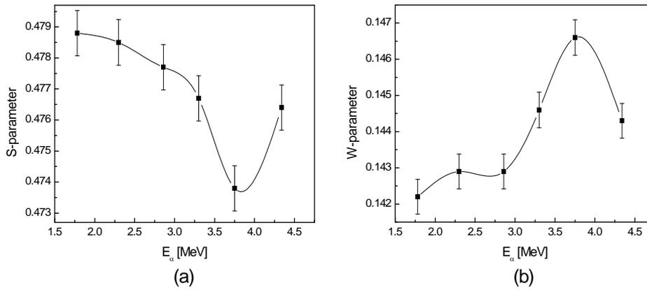
**Fig. (4):** The behavior of the S-parameter (a) and W-parameter (b) as a function of  $\alpha$ -particle energies at constant flux.
