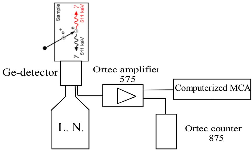
Fig. (1): Experimental setup for Doppler broadening line-shape measurements.
