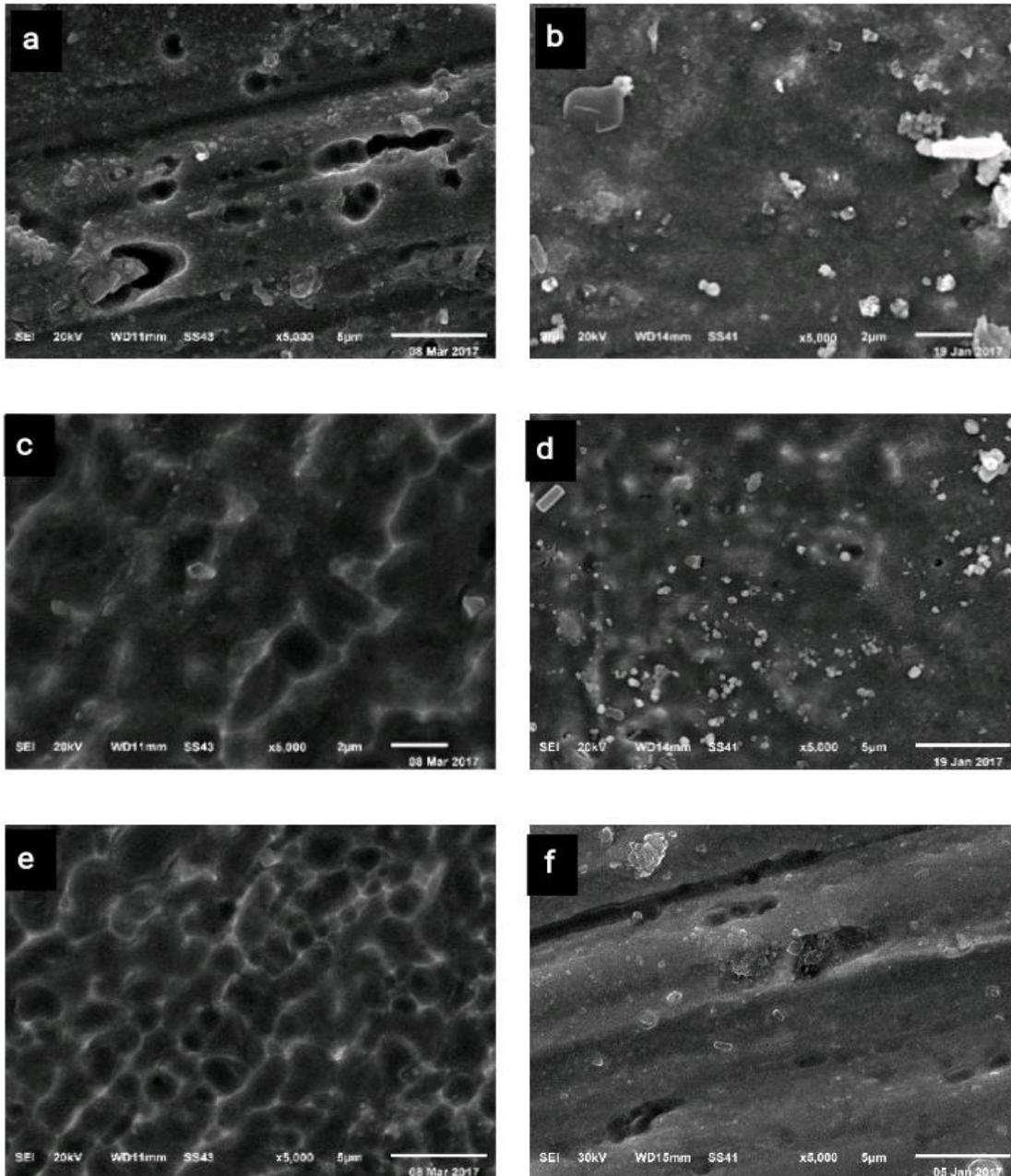
**Fig.2:** SEM images of Cu NiTi specimens after immersion in the testing solutions. a- Control      b- Cipro      c-Clotmazol
