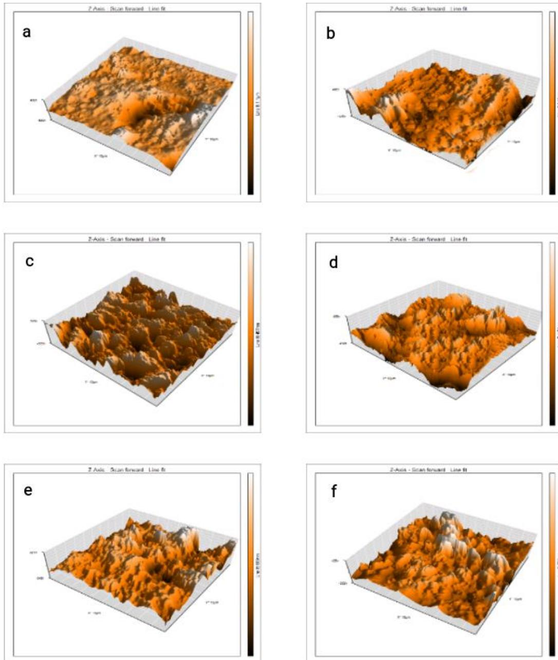
**Fig. 1:** AFM images of Cu NiTi arch wires after immersion in the testing solutions. a- Control      b- Cipro
