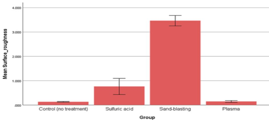
**Fig.1.** Means and standard deviations of the tested groups' surface roughness ( $\mu\text{m}$ ).
