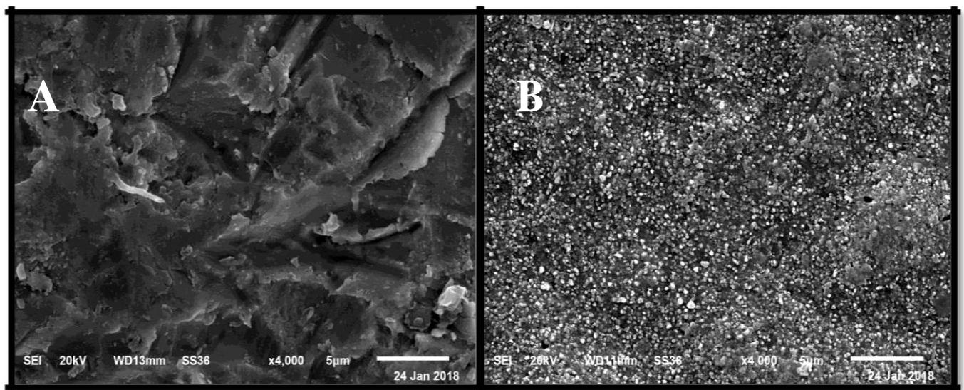
**Figure (1): A) SEM imaging at ×4000 magnification of zirconia surface after sandblasting treatment.****B) SEM imaging at ×4000 magnification of zirconia surface after etching by NH<sub>4</sub>HF<sub>2</sub>**
