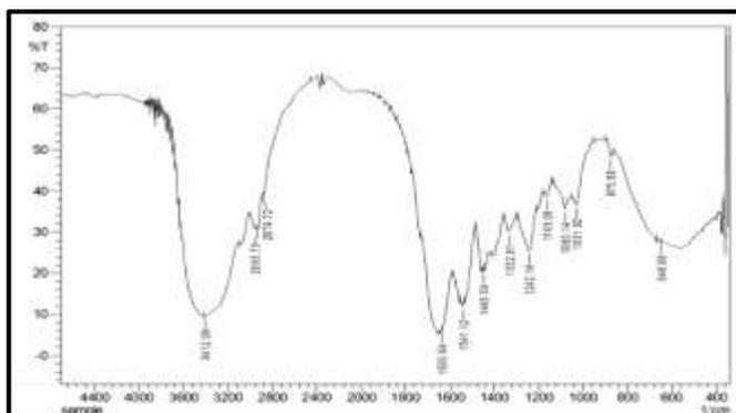
**Fig 7 FTIR analysis of the previous filling materials**
