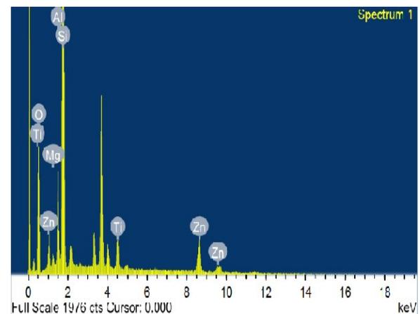
Fig. 4 (c) EDS spectrum of TiO<sub>2</sub> – coated glazed tile.
