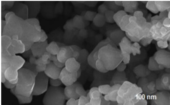
Fig.(2) SEM images for as- prepared TiO<sub>2</sub> nanoparticles .
