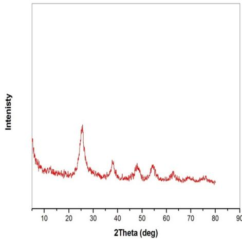
Fig. (1). XRD spectra of TiO<sub>2</sub> nanoparticles.
