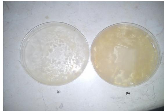
Fig. 6 Bacterial growth on nutrient agar for cultures taken from tile surfaces of TiO<sub>2</sub>- treated (a) and untreated (b) glazed tiles.
