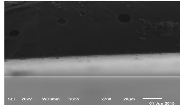
Fig. 4(b).SEM cross-section images of TiO<sub>2</sub> – coated glazed tile.
