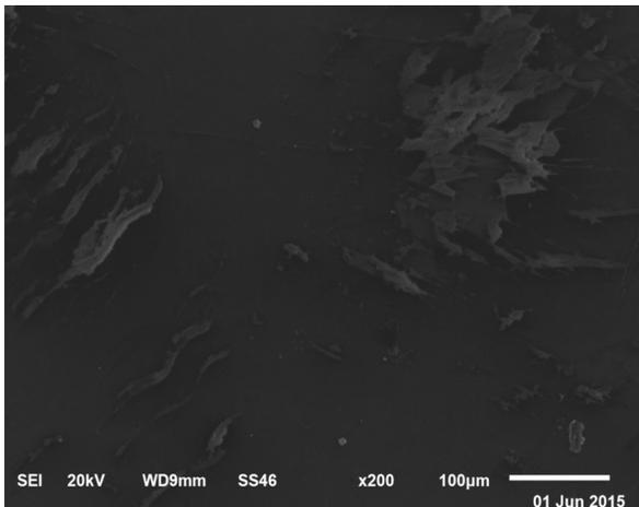
Fig.3 SEM surface images of TiO<sub>2</sub> coating.
