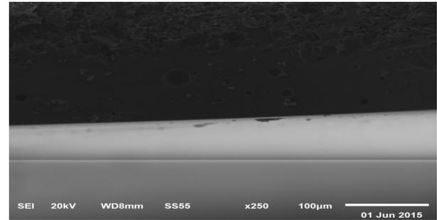
Fig. 4(a).SEM cross-section images of TiO<sub>2</sub> – coated glazed tile.
