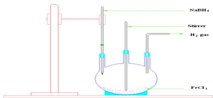
**Fig. (1)** Schematic diagram for synthesis of iron nanoparticles.
