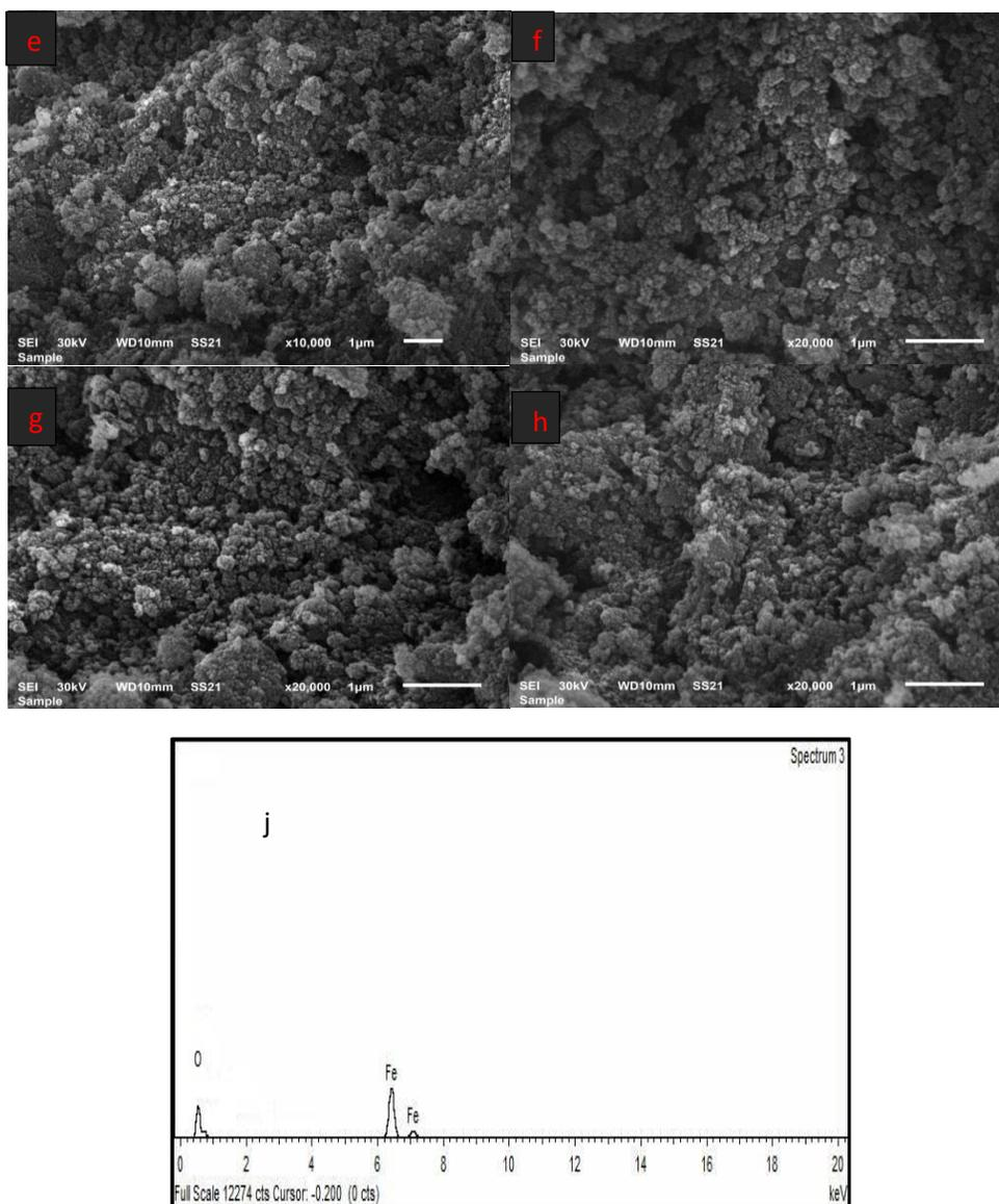
**Fig. (4)** FE-SEM images of the nZVI nanoparticles (Y (e-h), sample) and EDX pattern (j (Y)).
