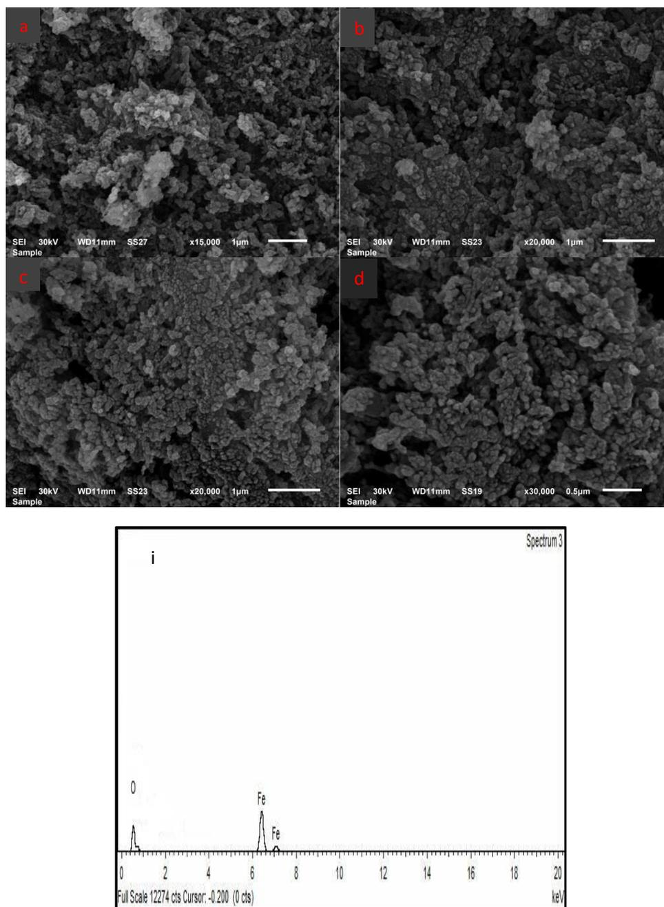
**Fig. (3)** FE-SEM images of the nZVI nanoparticles (X (a-d), sample) and EDX pattern (i (X)).
