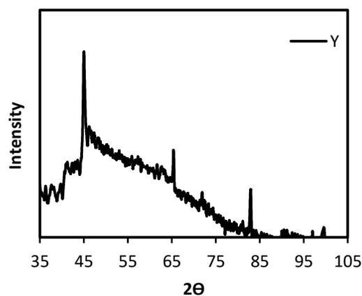
Fig. (2b) X-ray diffraction (XRD) pattern of Y.
