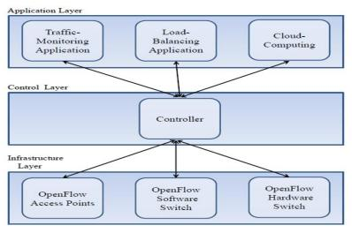
Fig (1) Three layers of SDN structure.
