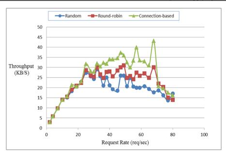
Fig (6) Request rate vs Throughput using Raspberry Pi
