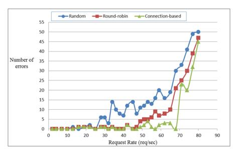
Fig (7) Request rate vs Number of errors using Raspberry Pi.
