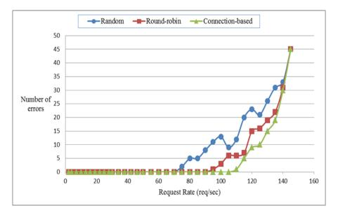
Fig (5) Request rate vs Number of errors using mininet
