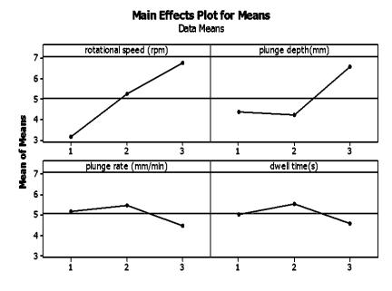
Fig (4) Main effects of means for tensile-shear strength
