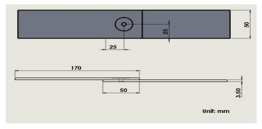
Fig (2) The tensile-shear specimen. (Dimensions in mm)
