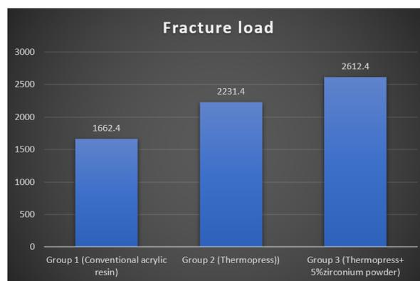
Figure (3): Bar chart representing fracture load for different groups
