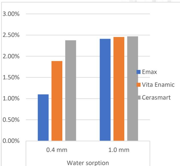
**Figure 3: Bar chart showing average water sorption (%) for different materials and thicknesses**
