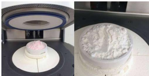
**Figure 1: removing the food dye from the ceramic powder**
