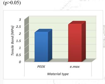
**Figure (4):** Column chart showing the mean values of tensile bond strength for both material groups
