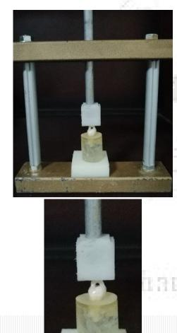
Figure (3): cementation of endocrown using the cementation device.
