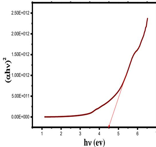
Fig. 4. The relation between  $(\alpha h\nu)^2$  and  $h\nu$  for the obtained ZnS Nanoparticles.
