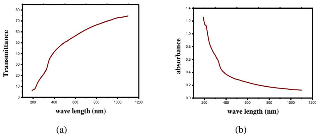
Fig. 3. (a) The transmission spectrum (b) The absorption spectrum of the synthesized ZnS nanoparticles
