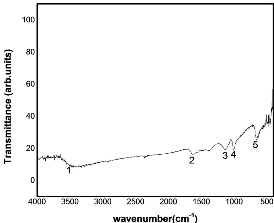
Fig. 6. FTIR spectrum of ZnS nanocrystals
