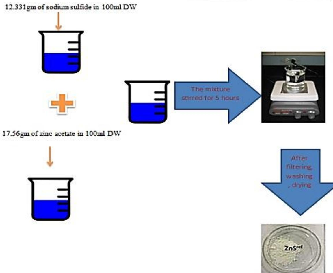
Fig 1. Schematic representation of the chemical precipitation procedure of ZnS nanoparticles
