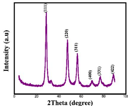
Fig 2.X-ray diffraction patterns of ZnS
