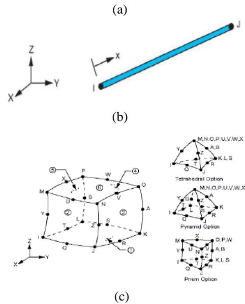
Figure 15: Different elements using in the FEM. (a) Solid 65, (b) Link 180, (c) Solid 185 [40]
