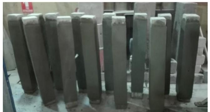
Figure 5: Column specimens after applying ferrocement jacket.
