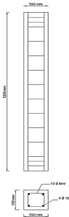
Figure 1: Concrete columns details.
