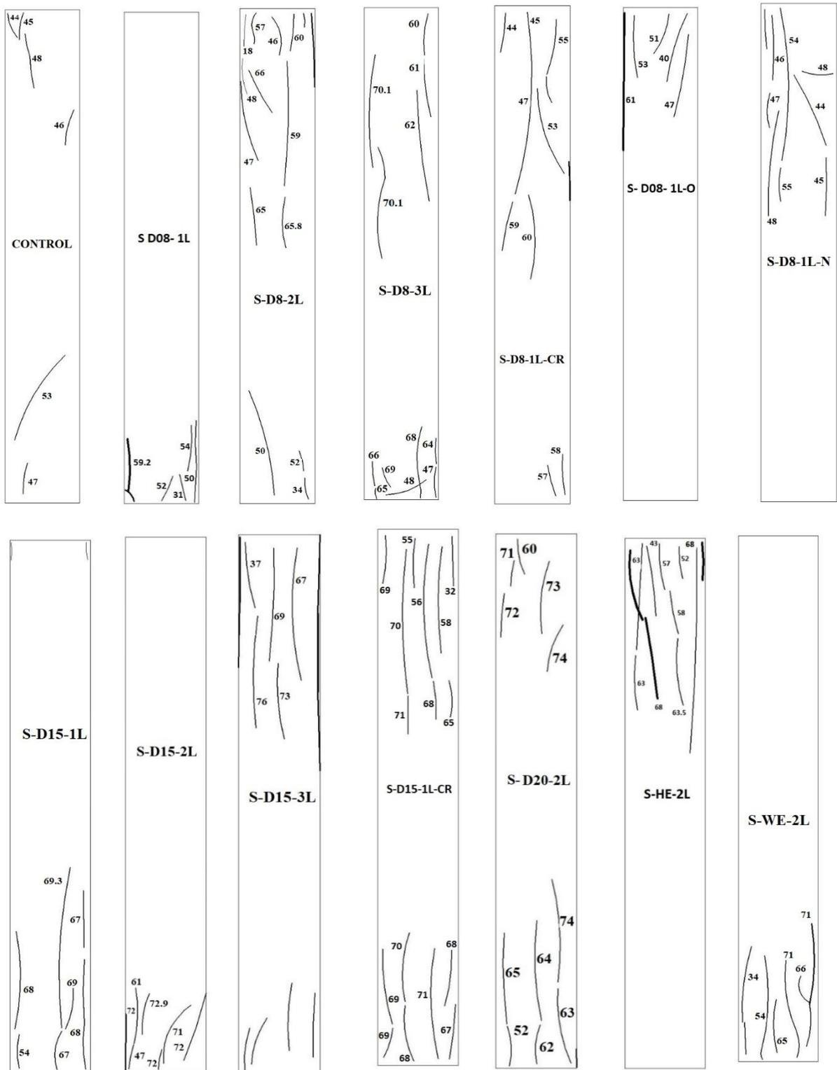
Figure 10: Schematic representation of cracking patterns at failure.
