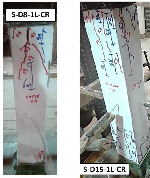
Figure 9: Cracking pattern at failure for specimens S-D8-1L-CR and S-D15-1L-CR
