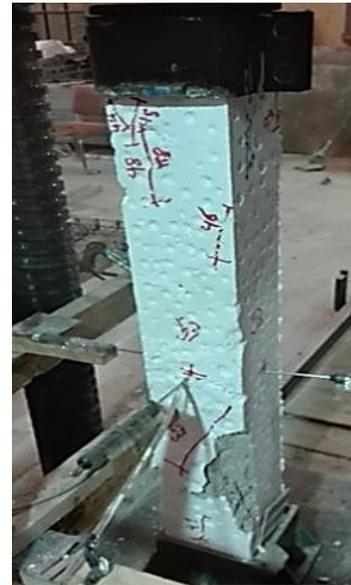
Figure 7: Cracking pattern at failure for control specimen SC
