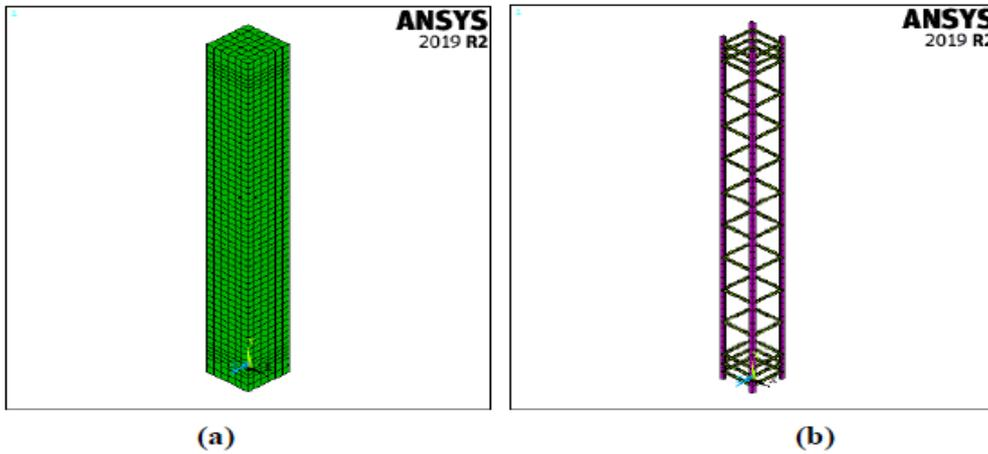
Figure 16: Model used for the control specimen SC. (a) concrete mesh, (b) reinforcing steel bars.
