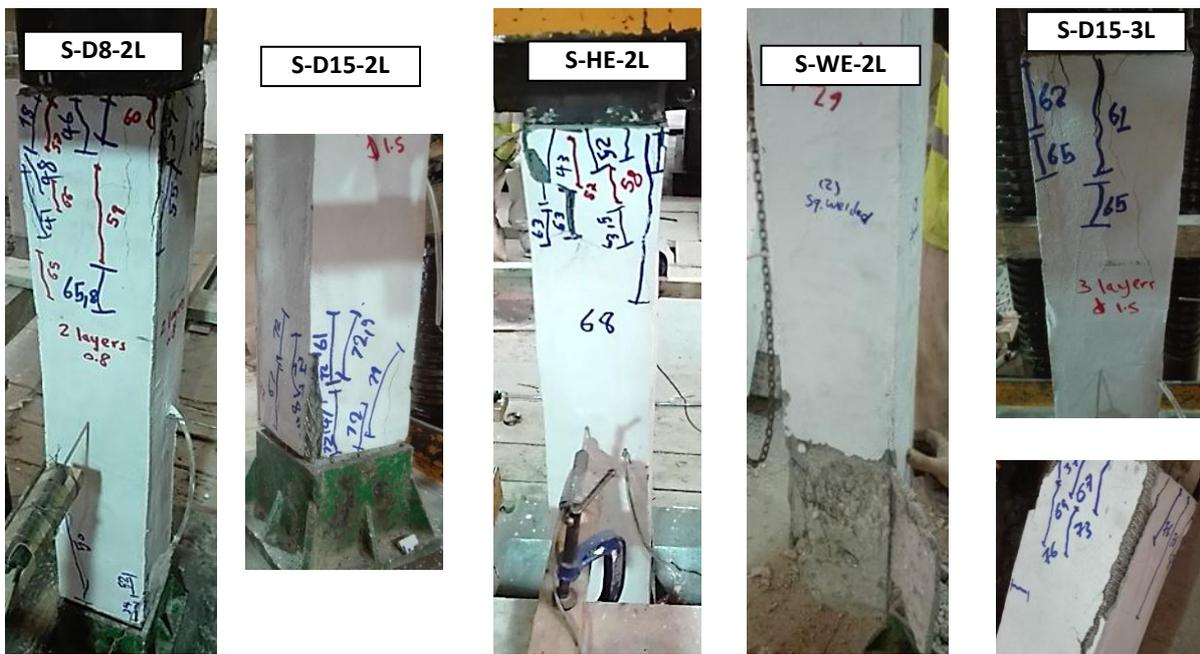
Figure 8: Cracking pattern at failure for sample strengthened specimens
