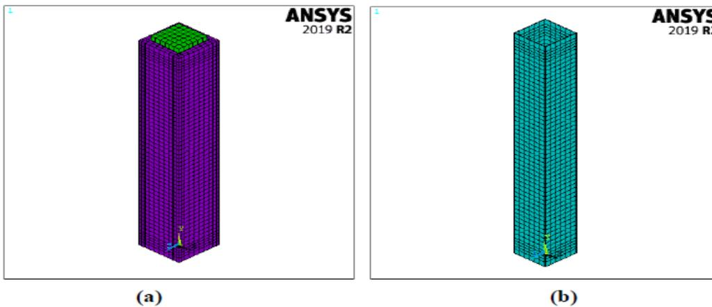
Figure 17: Model used for the strengthened specimens. (a) Concrete and mortar mesh, (b) Wire layer mesh.
