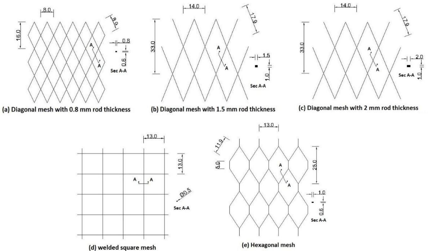
**Figure 3: The Five different types of steel mesh used.**
