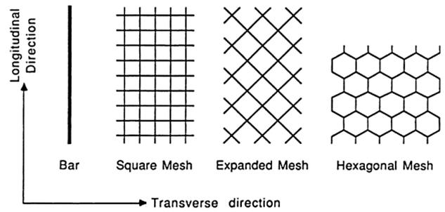
Figure 20: Proposed longitudinal and transverse directions of reinforcement mesh [2].
