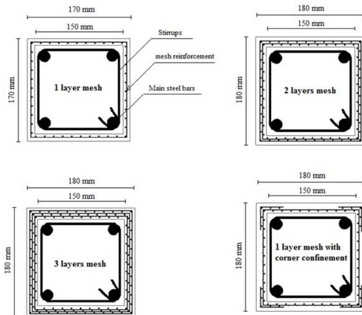
Figure 2: Different ferrocement jackets used for strengthened specimens.
