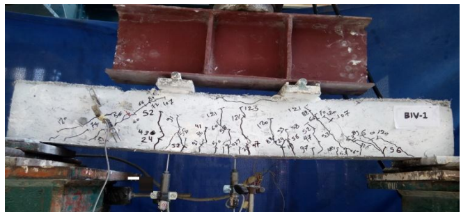
Fig. 10: Final crack pattern of beam BIV-1.
