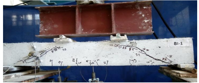
Fig. 7: Final crack pattern of beam BI-1.
