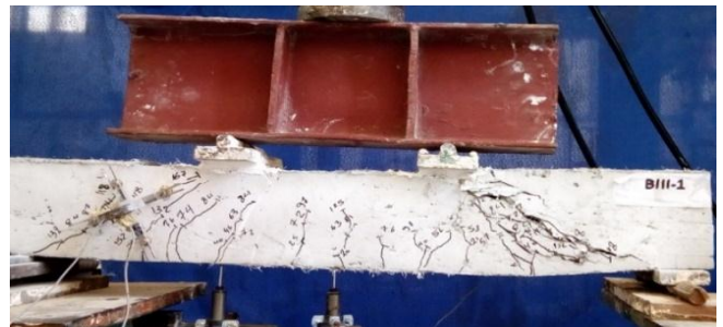
Fig. 9: Final crack pattern of beam BIII-1.
