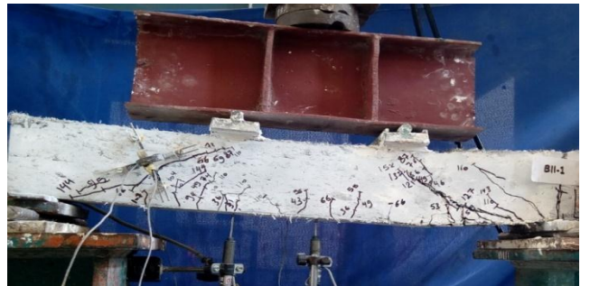
Fig. 8: Final crack pattern of beam BII-1.
