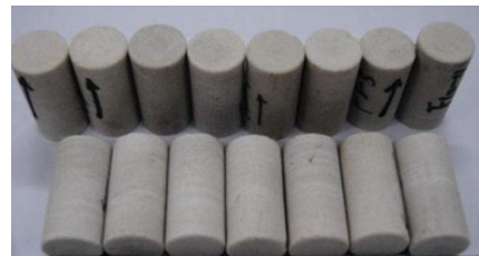
Figure 5. Shape of the Cylindrical Samples of Marble rocks
