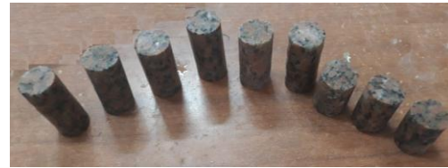
Figure 2. Shape of the Cylindrical Samples of Aswan Granite rocks
