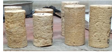
Figure 3. Shape of the Cylindrical Samples of Sandstone rocks
