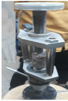
Figure 6. Point Load Test System
