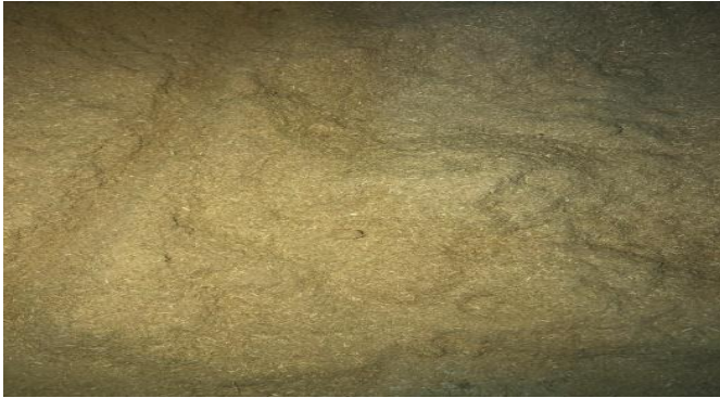
Figure 2 Mechanically fibrated rice straw fibers
