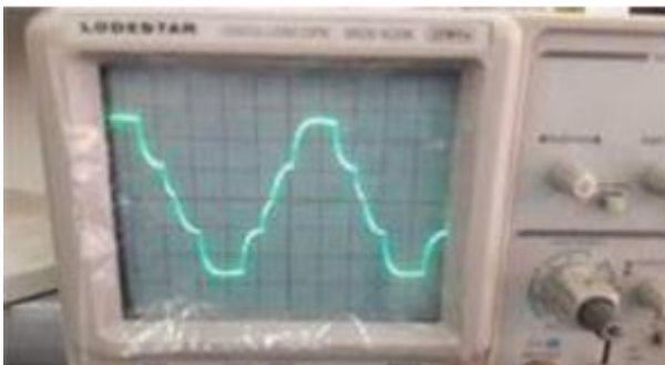
Fig.12 Line to line output voltage waveform at the secondary side of main transformer.
