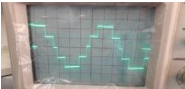
Fig. 11. Line to line output voltage waveform at the primary side of main transformer
