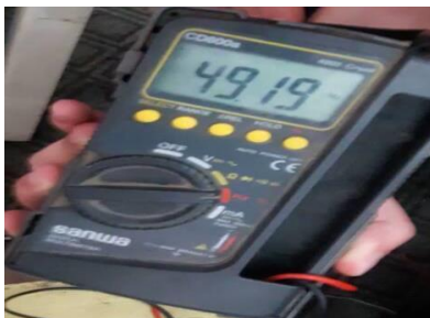
Fig.13 The three level H bridge inverter output frequency.
