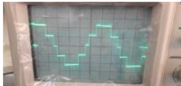
Fig. 16. Line to line output voltage waveform at the primary side of main transformer for the second case operating condition.
