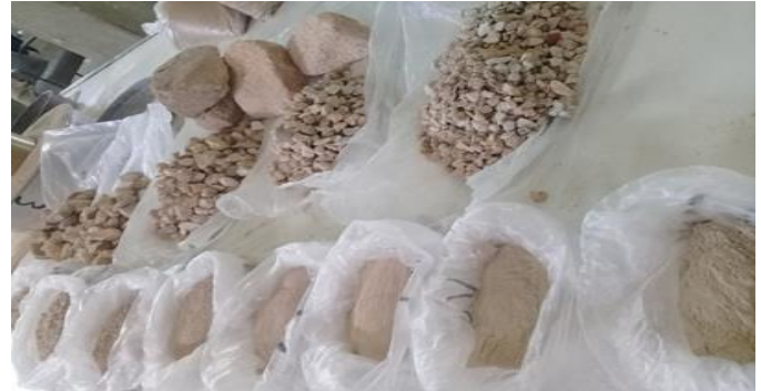
Figure 1. Graded recycled refractory brick
