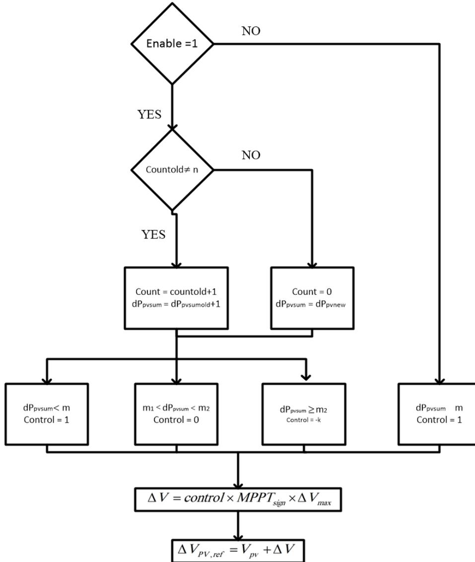
**Fig 5** Flow chart of power ramp rate control by modified MPPT
