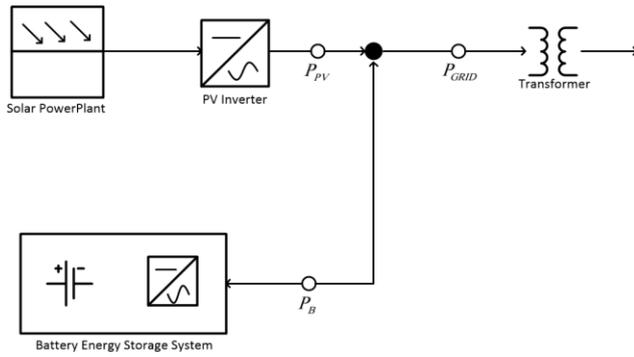
**Fig. 2** Schematic of a PV power plant generation and a connected BESS to grid
