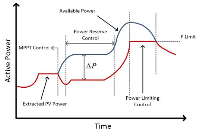
**Fig. 1** Three different active power control schemes action times
