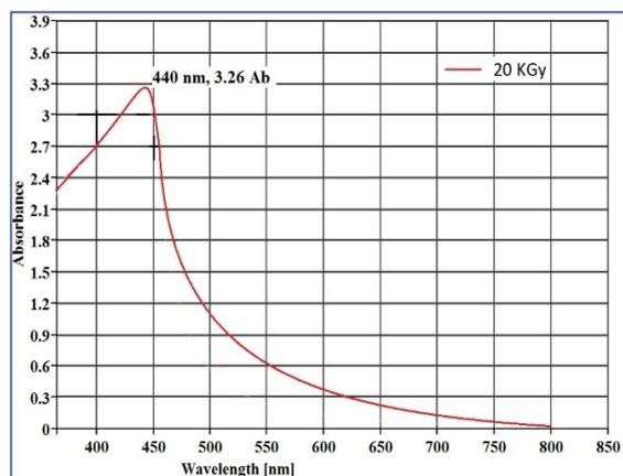
**Figure (1):** Uv-Vis. Spectroscopy of AgNPs synthesized by gamma irradiation (20.0 kGy) and PVP.
