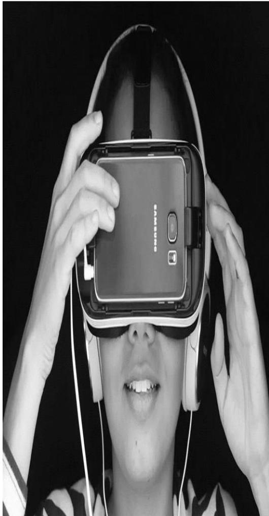
**Fig.2.** Virtual Reality Goggles Attached with Smart Phone and Headset with Headphones
