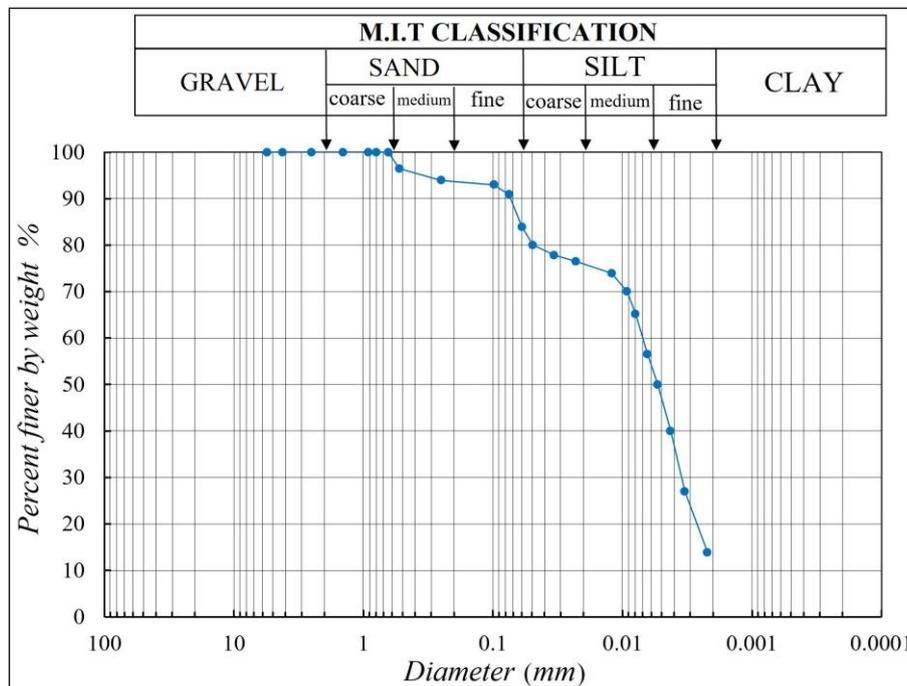
Figure 1. Grain size distribution for the expansive soil
