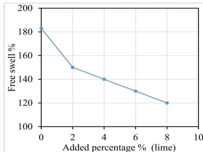
Figure 9. Variation of free swell values for different lime content
