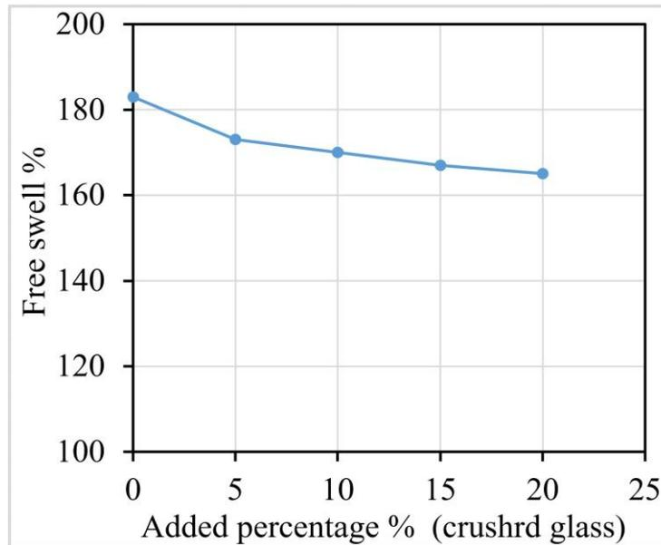
Figure 8. Variation of free swell values for different crushed glass wastes content
