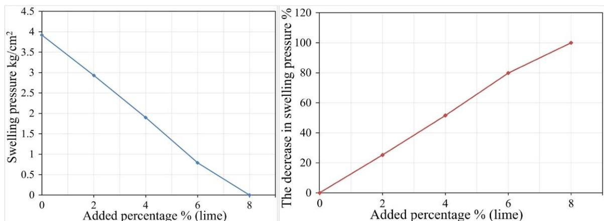
Figure 11. The effect of adding lime on the swelling pressure
