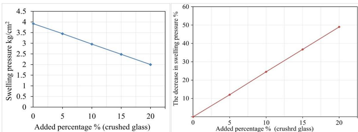
Figure 10. The effect of adding crushed glass wastes on the swelling pressure
