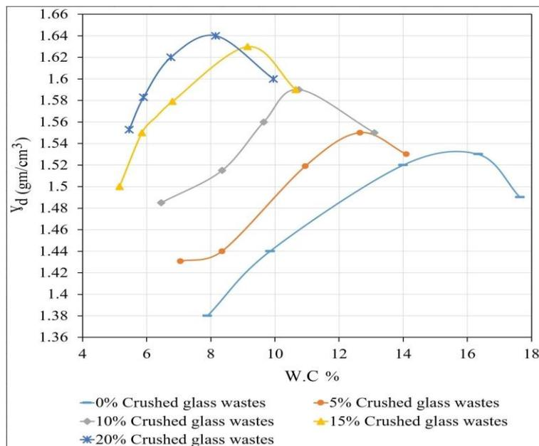
Figure 4. Compaction tests curves of the expansive soil-crushed glass wastes mixtures
