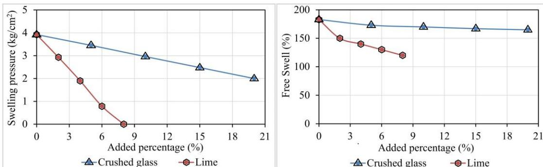
Figure 17. The comparison between the effect of adding crushed glass wastes and lime separately on soil's swelling properties
