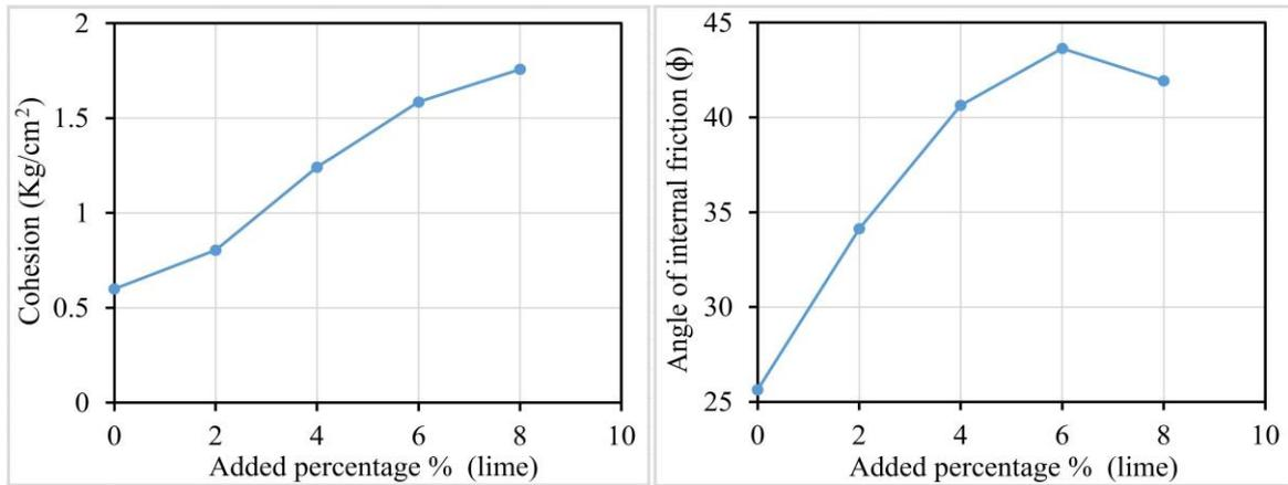
Figure 7. Variation of the shear parameters values against the percentage of added lime
