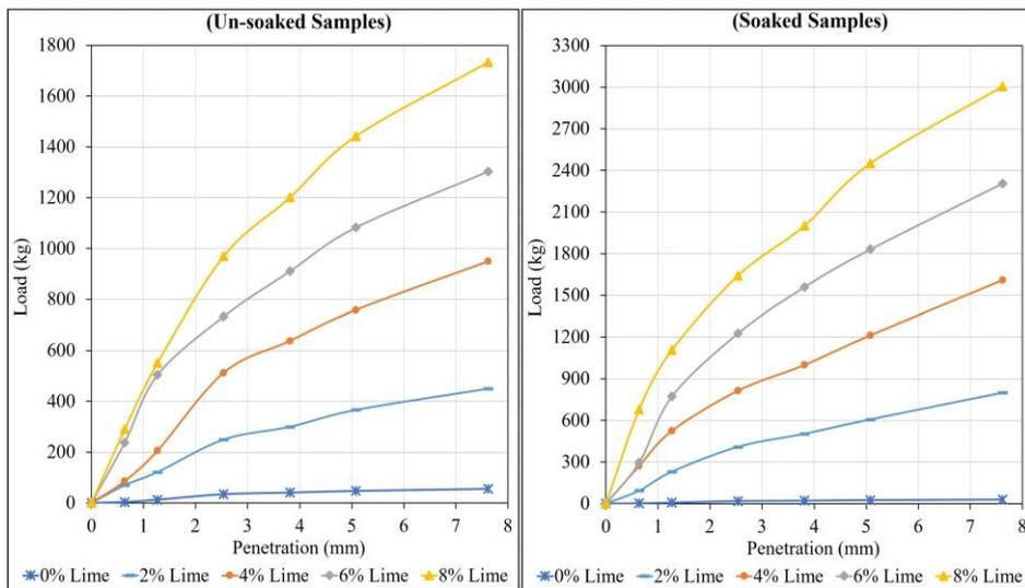
Figure 15. The penetration-load curves of the expansive soil-lime mixtures based on un-soaked/ soaked CBR tests
