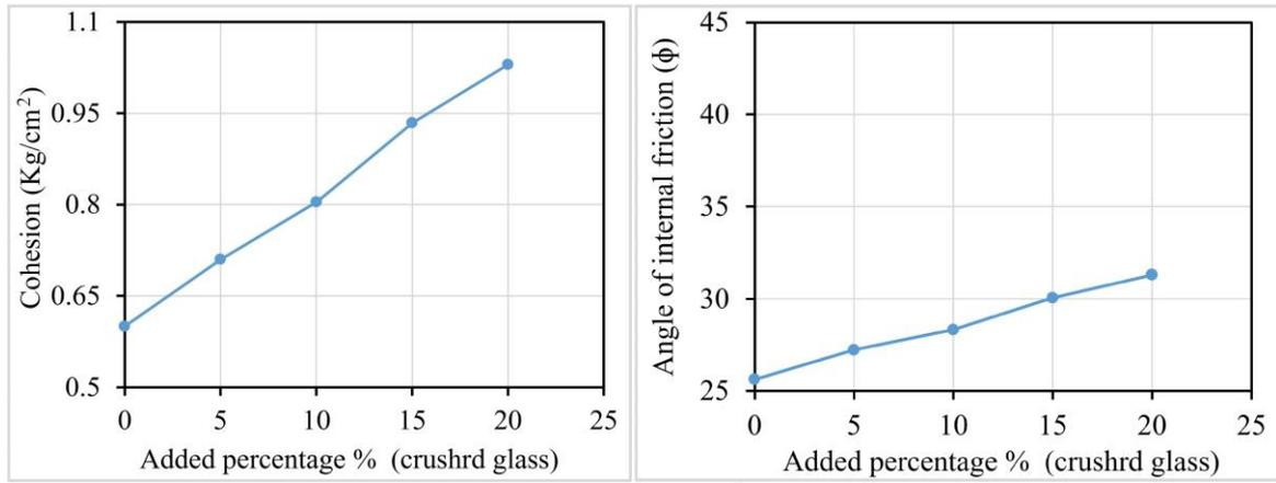
Figure 6. Variation of the shear parameters values against the percentage of added crushed glass
