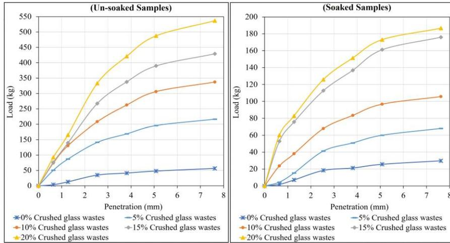
Figure 13. The penetration-load curves of the expansive soil-crushed glass wastes mixtures based on un-soaked/ soaked CBR tests
