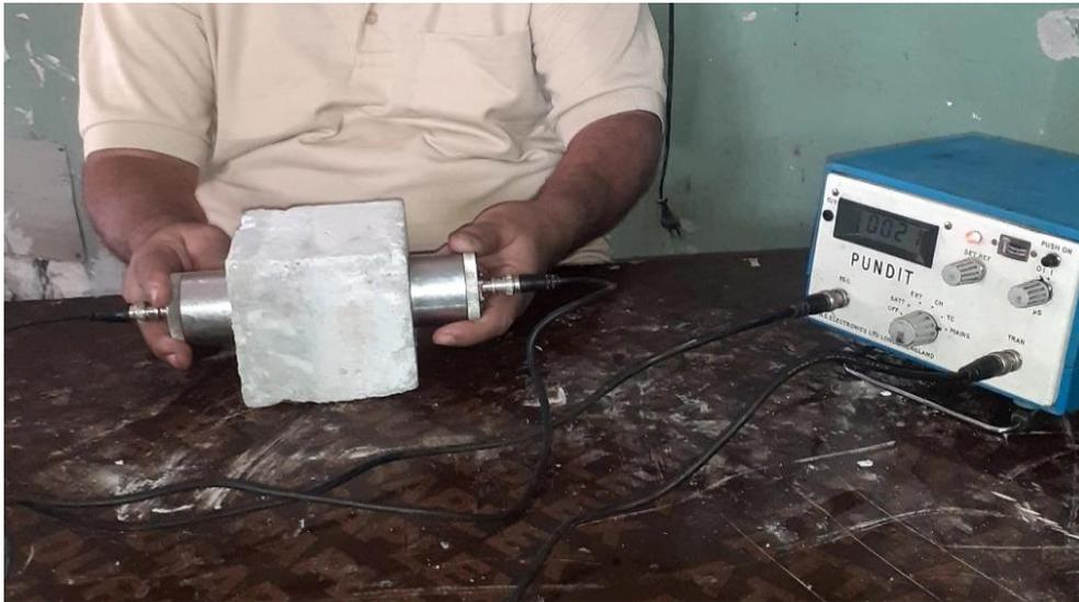
Fig. 4: Experimental Set-up for Ultrasonic Pulse Velocity Testing
