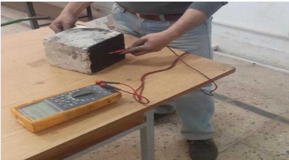
Fig. 3 Experimental Set-up for Electrical Surface Resistivity Testing
