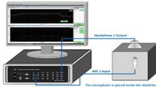
Fig. 6. Photograph for hardware connection of MEMS speaker-test
