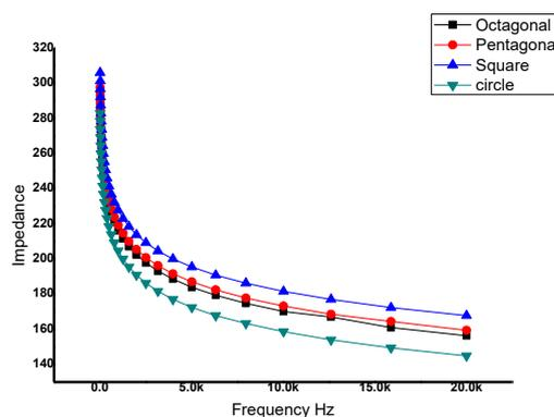
Fig. 5. Simulated results for impedance versus frequency for different geometries.
