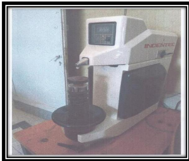
**Fig. (3)** Rockwell testing machine
