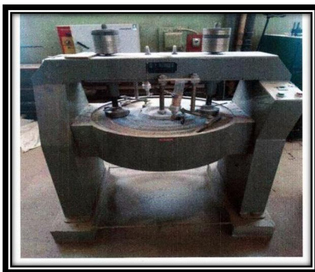
Fig. (5) Abrasion test machine
