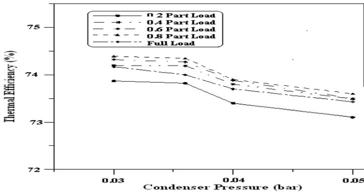
Fig. 8: Effect of Condenser Pressure on Thermal Efficiency
