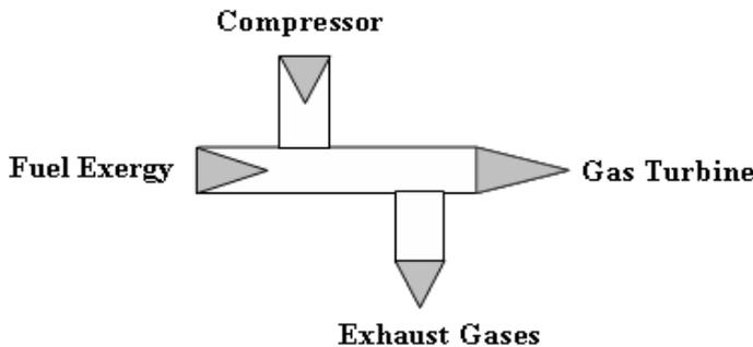
Fig. 3: Exergy Balance in Gas Power Plant
