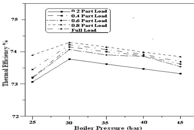
Fig 6: Effect of Live Steam Pressure on Thermal Efficiency
