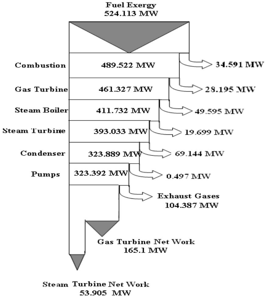
Fig. 4: Component Exergy Flow Chart of Combined Cycle
