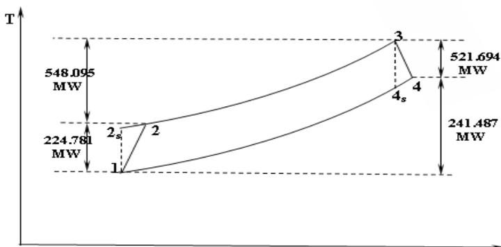
Fig. 5: First Law Heat Balance of Gas Power Plant
