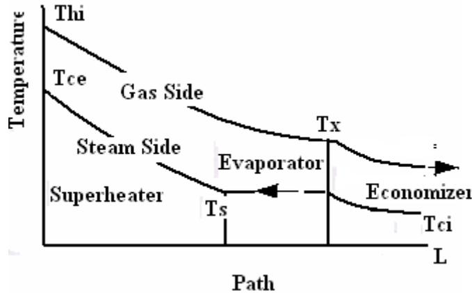
Fig. 2: Temperature Variation Along the Waste Heat Boiler Paths
