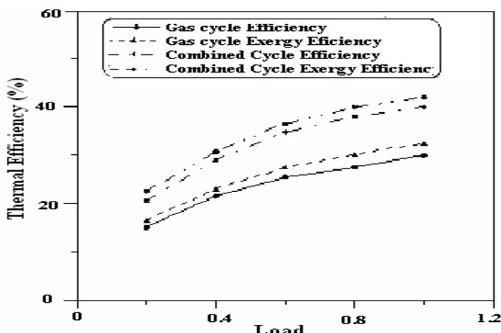
Fig. 9: Comparison between Different Cycles and Thermal Efficiency
