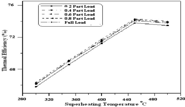
Fig. 7: Effect of Live Steam Superheating Temperature on Thermal Efficiency
