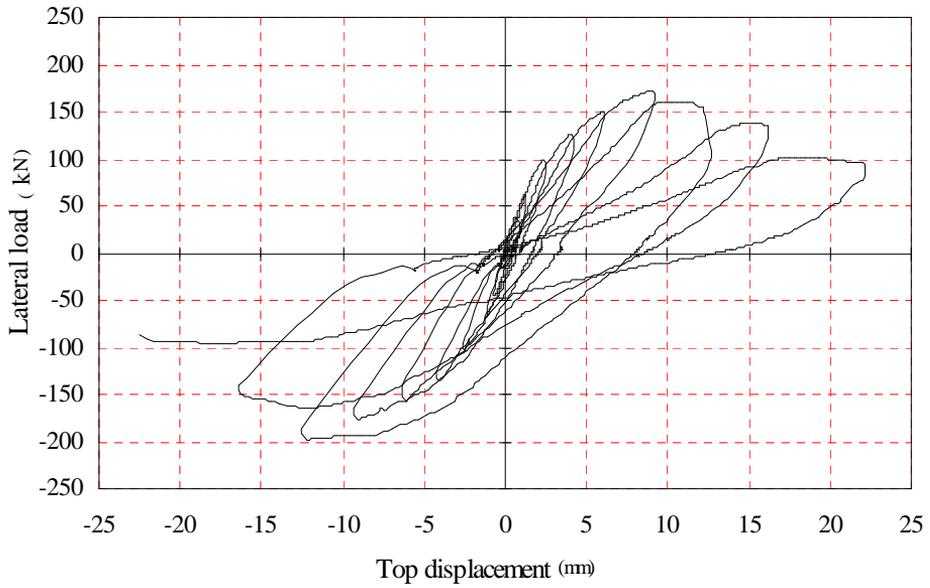
Fig. (5) Cyclic load and displacement of specimen HL – 2
