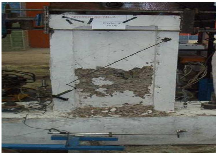
Fig. (11) Crack pattern of specimen HL-2
