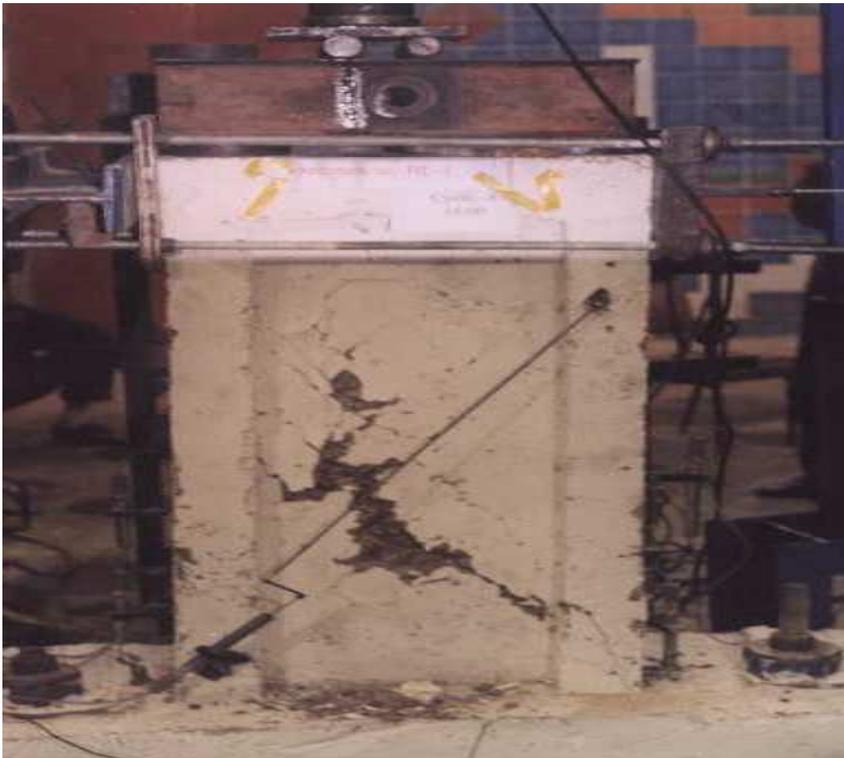
Fig. (10) Crack pattern of specimen HL-1
