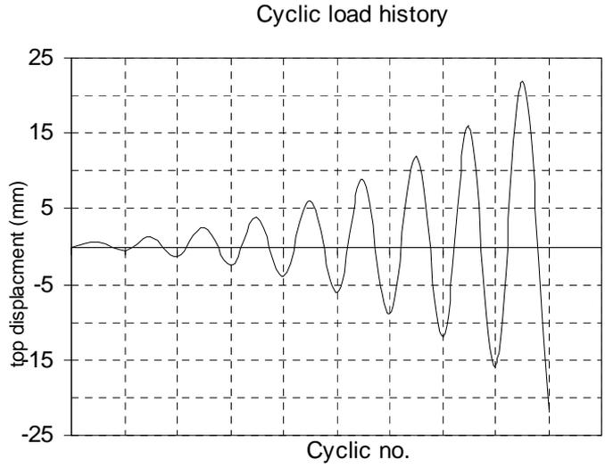
Fig. (3) Cyclic load history used for tests
