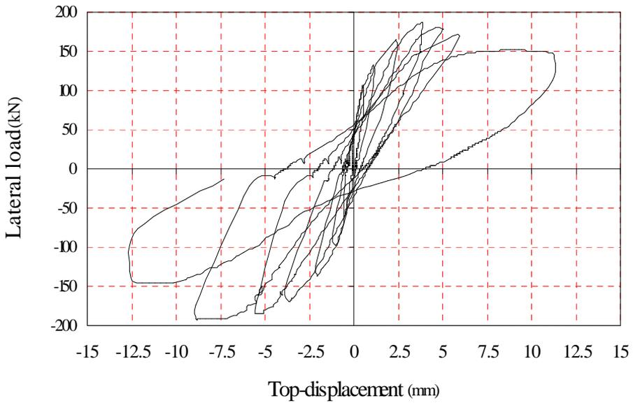
Fig. (8) Cyclic load and displacement of specimen NL
