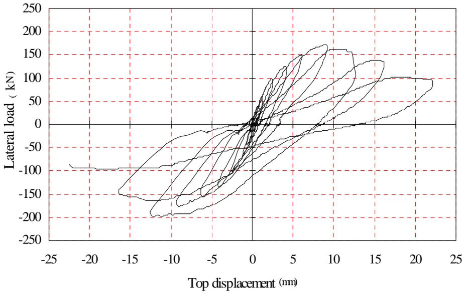
Fig. (7) Cyclic load and displacement of specimen HS – 2
