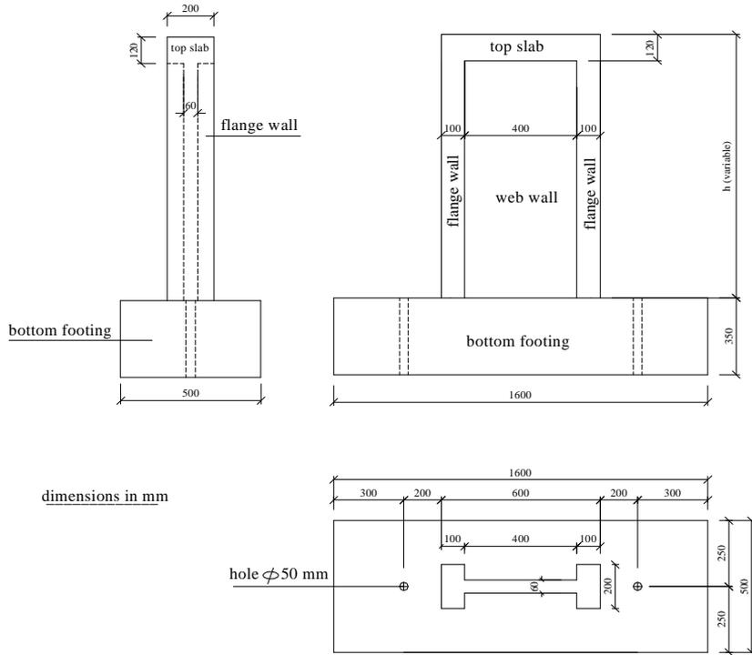
Fig. (1) Dimensions of the tested long walls
