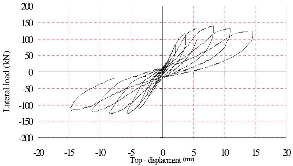
Fig. (9) Cyclic load and displacement of NS
