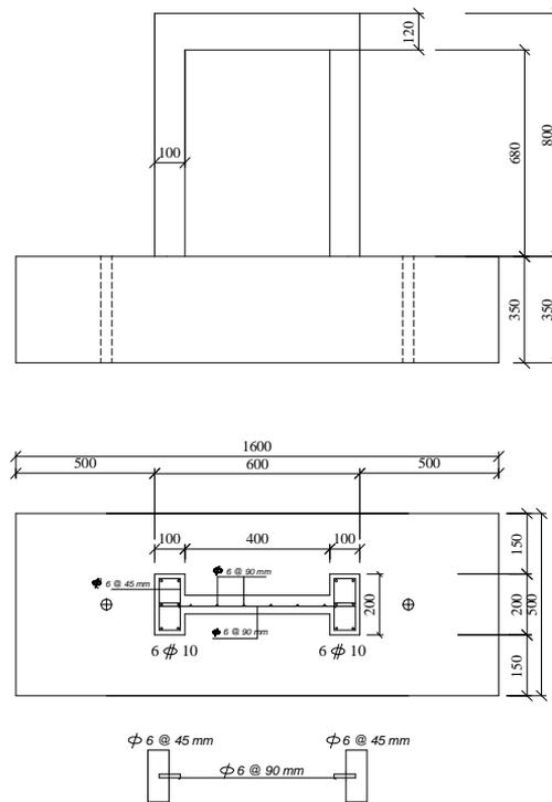
Fig. (2) Reinforcement details
