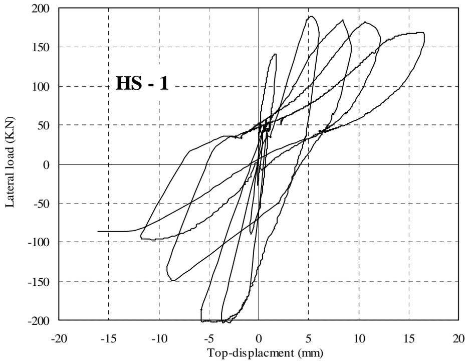
Fig. (6) Cyclic load and displacement of specimen HS – 1
