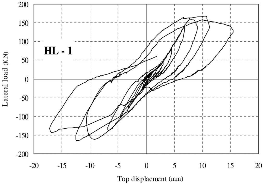
Fig. (4) Cyclic load and displacement of specimen HL – 1
