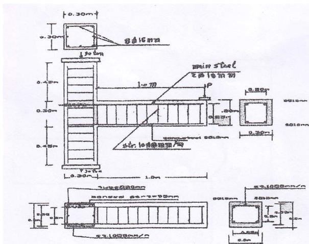
Fig. (1) : Cantilever-to-column connection specimens.
