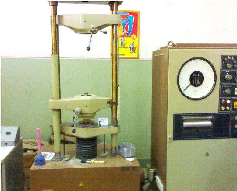
Fig. (10) Photo of the Brazilian indirect tension test machine
