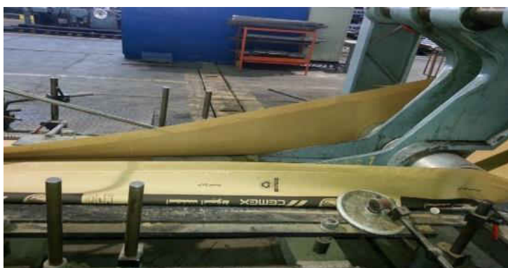
Fig. 7. First steps in sacks forming (overlapping)
