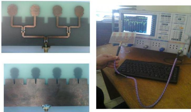
**Fig. 39.** The fabricated photos of the proposed 4 x 1 UWB linear antenna array.
