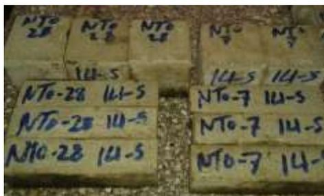
**Fig. 4.** Cement Mortar Specimens Incorporating NT
