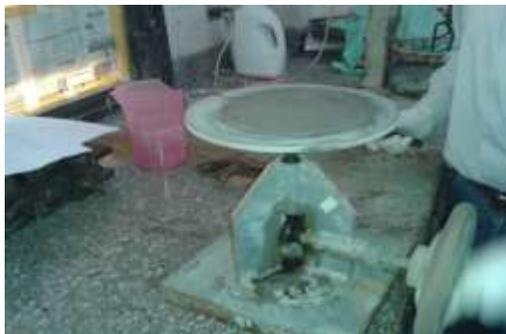
**Fig. 5.** Flow Table Test
