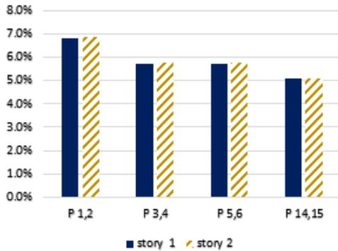
Fig. 14. % Difference of story drift of building with openings at first and second stories compared with that without opening.
