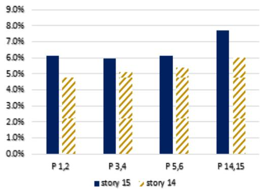
Fig. 17. % Difference of story drift of building with openings at fourteenth and fifteenth stories compared with that without opening.
