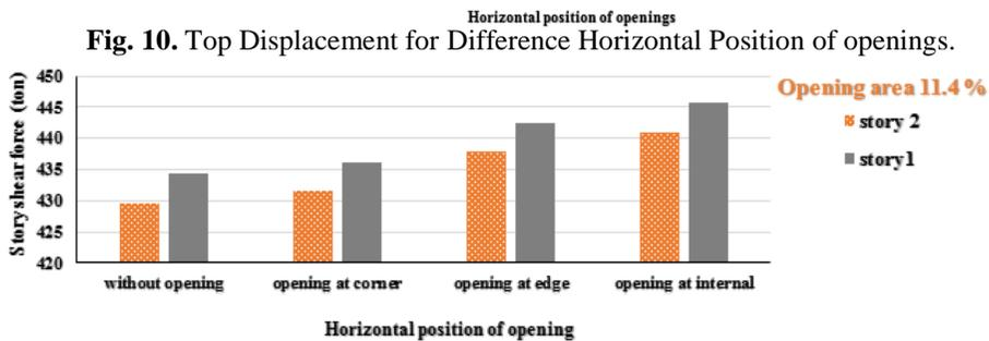
Fig. 11. Story Shear Force for difference Horizontal Position of openings.
