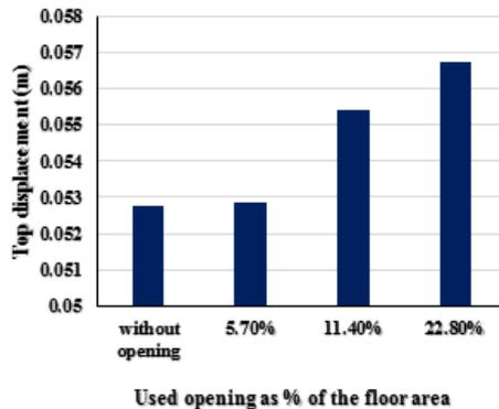
Fig. 7. Top Displacement for Difference Area of Openings.
