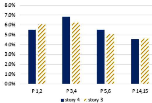
Fig. 15. % Difference of story drift of building with openings at third and fourth stories compared with that without opening.
