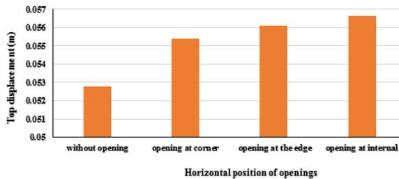
Fig. 10. Top Displacement for Difference Horizontal Position of openings.
