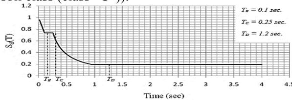
Fig. 2. Design Response Spectrum Used in the Analysis.
