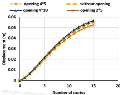
Fig. 6. Maximum Displacement for Difference Area of Openings.
