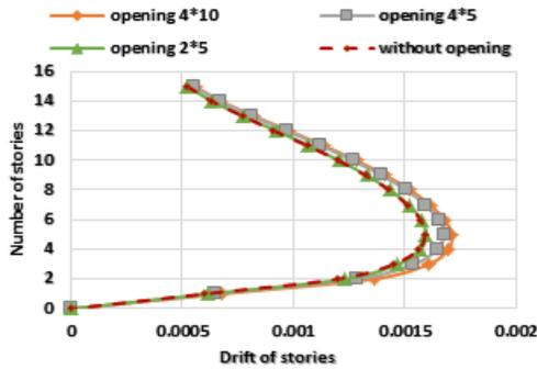
Fig. 4. Story Drift for Difference Area of Openings.
