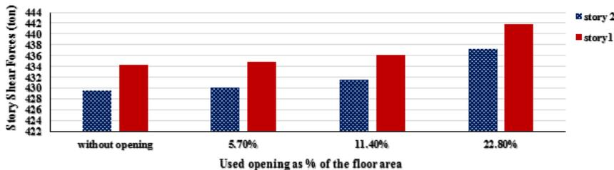
Fig. 8. Story Shear Force for Difference Area of Openings
