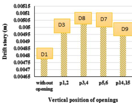
Fig. 12. Maximum Story Drift for Difference Vertical Position of openings.
