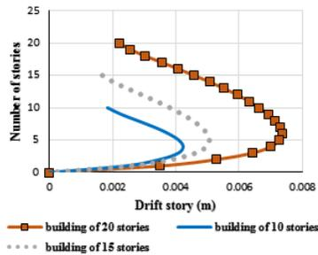
Fig. 19. Story Drift for Opening of Slab.
