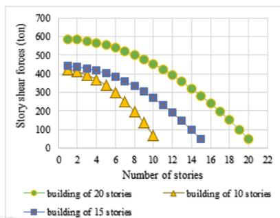
Fig. 23. Story Maximum Shear Force in X Direction.
