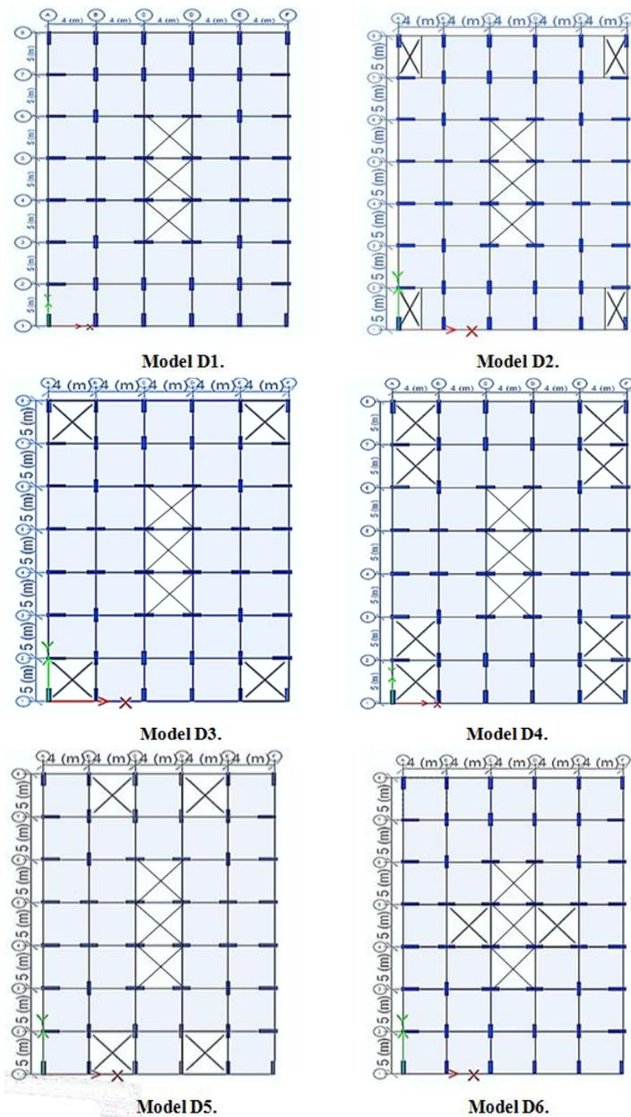
Fig. 3. Types of openings in the slab
