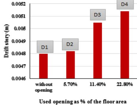
Fig. 5. Maximum Story Drift for Difference Area Openings.
