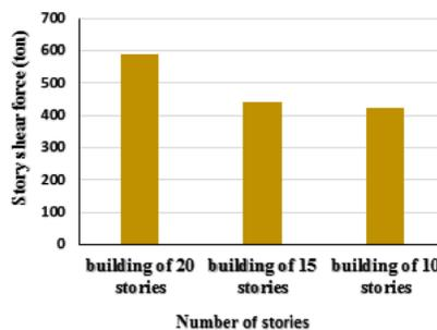
Fig. 24. Story Maximum Shear Force at first (Ground) level.
