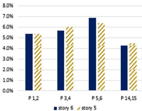
Fig. 16. % Difference of story drift of building with openings at fifth and sixth stories compared with that without opening.
