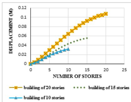
Fig. 21. Story Maximum Displacement in X Direction.
