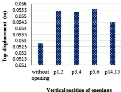
Fig. 13. Top Displacement for Difference Vertical Position for openings.
