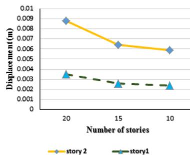
Fig. 22. Story Displacement Values at Openings Level.
