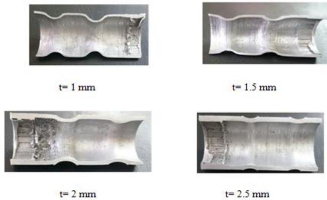
a- Photos of wall sections in throttling reduction.
