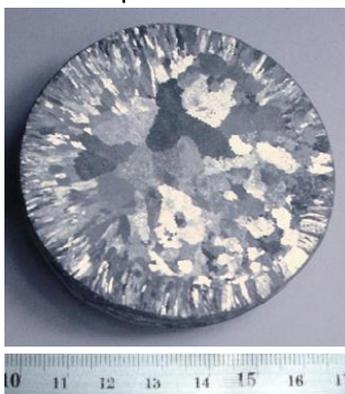
**Fig. 1.** Macrograph of unrefined aluminium specimen.
