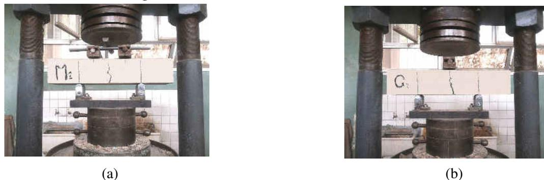
**Fig. 4.** The failure shape of beams in the two cases of loading, (a) Two third point loading, (b) center point loading.
