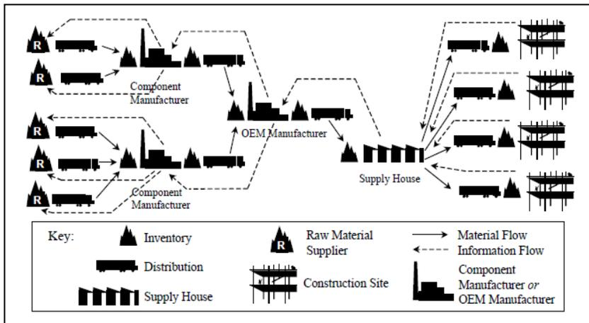
**Fig. 1.**Construction supply chain for building materials [7].
