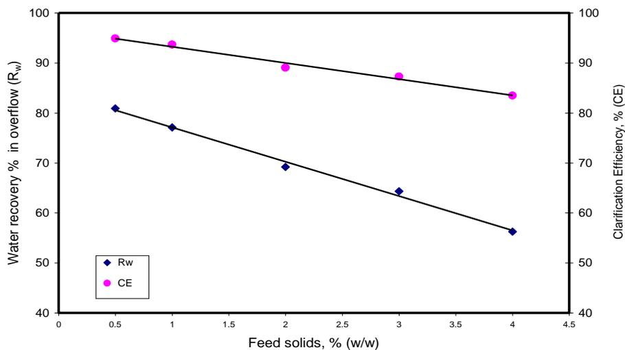
Fig .8 : The effect of feed concentration on water recovery & clarification efficiency of the whole system.
