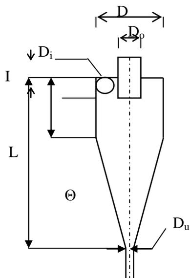
Fig. 2 : Illustration of the hydrocyclone geometry
