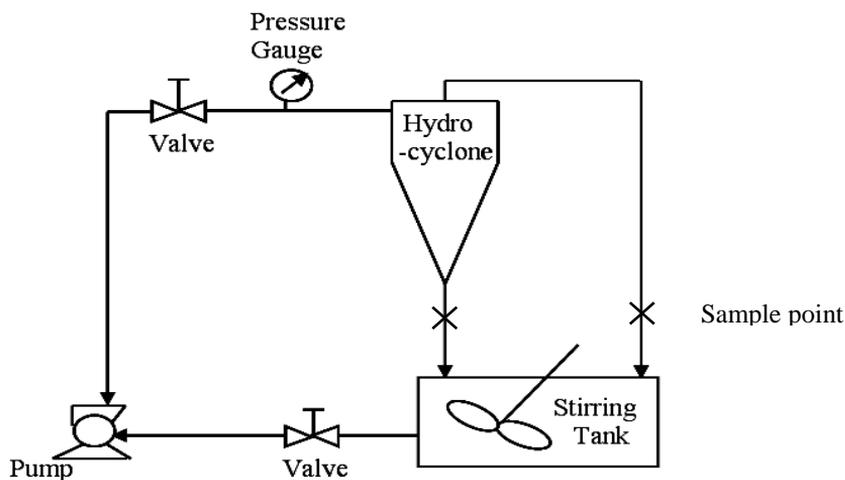
Fig. 3 : Schematic diagram of the experimental setup of single stage.
