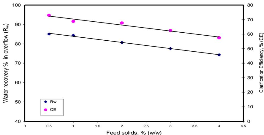
Fig .6 : The effect of feed concentration on water recovery and clarification efficiency of the first stage hydrocyclone .
