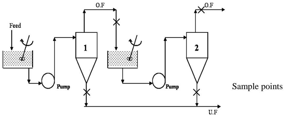
**Fig.4** : Two stage hydrocyclone in series connection
