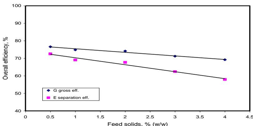
Fig .5 : The effect of feed concentration on overall efficiency of the first stage hydrocyclone.
