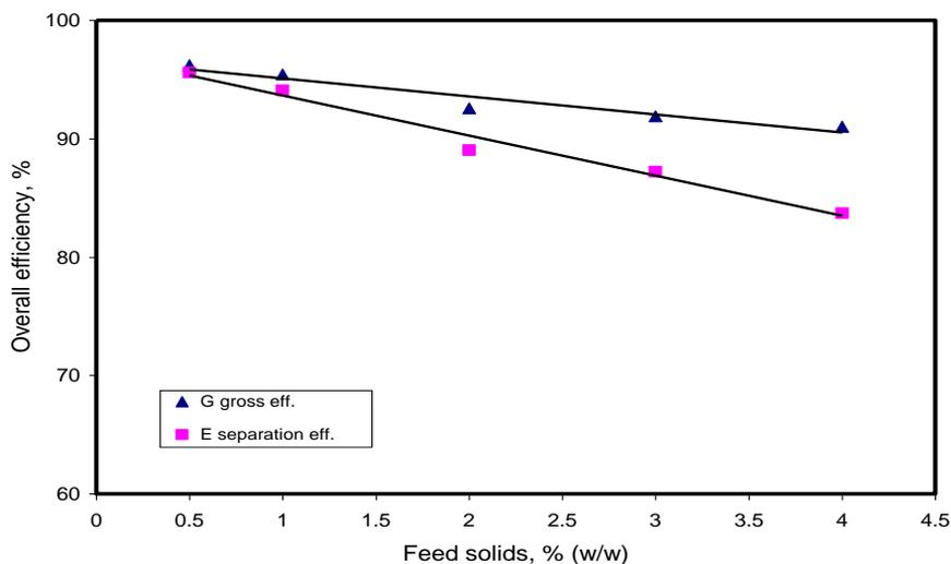
Fig. 7 : The effect of feed concentration on overall efficiency of the whole system.
