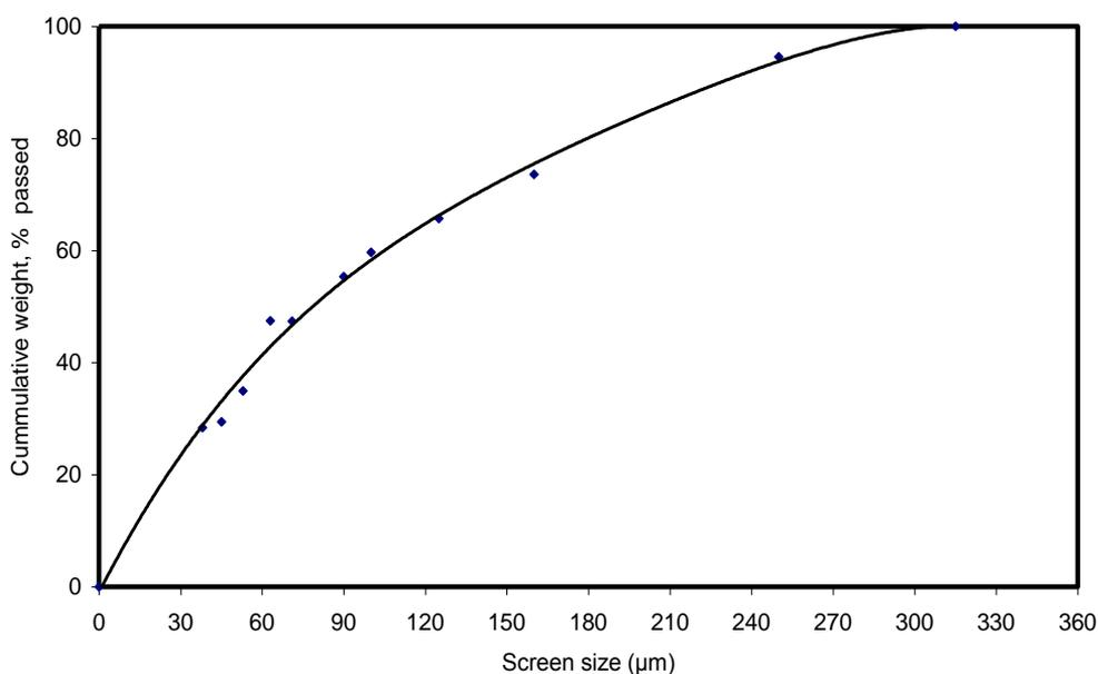
Fig. 1 : Particle size distribution of the sludge sample.
