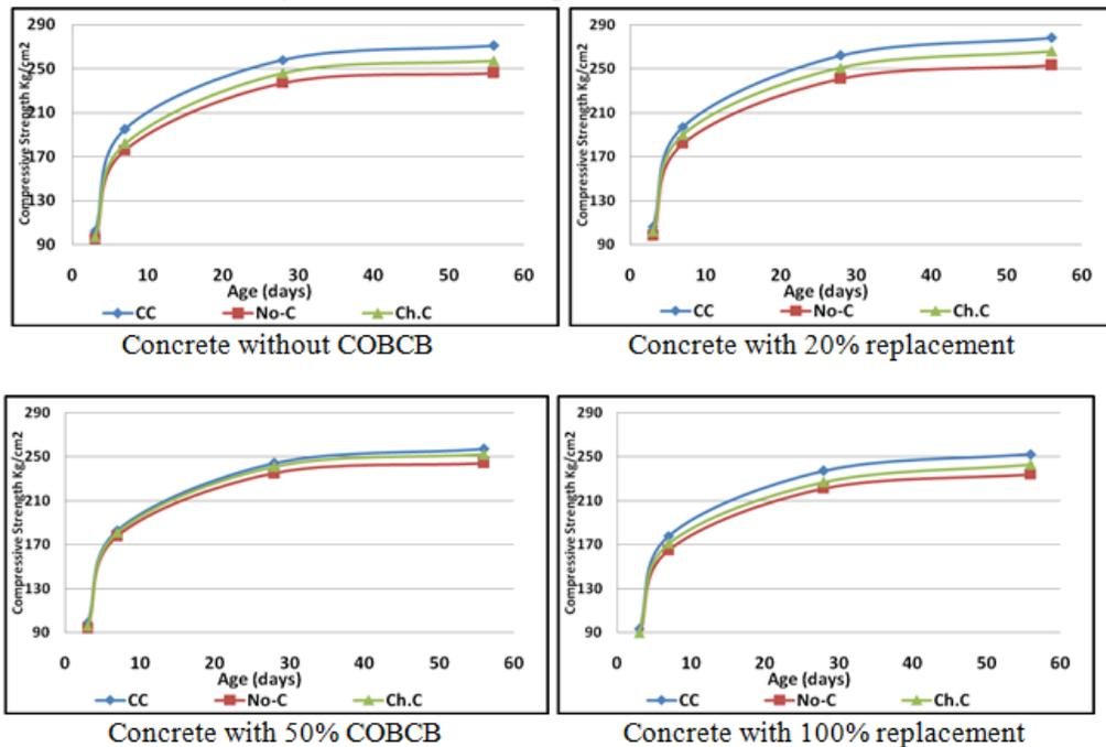
Fig. 7. Effect of curing type on compressive strength.
