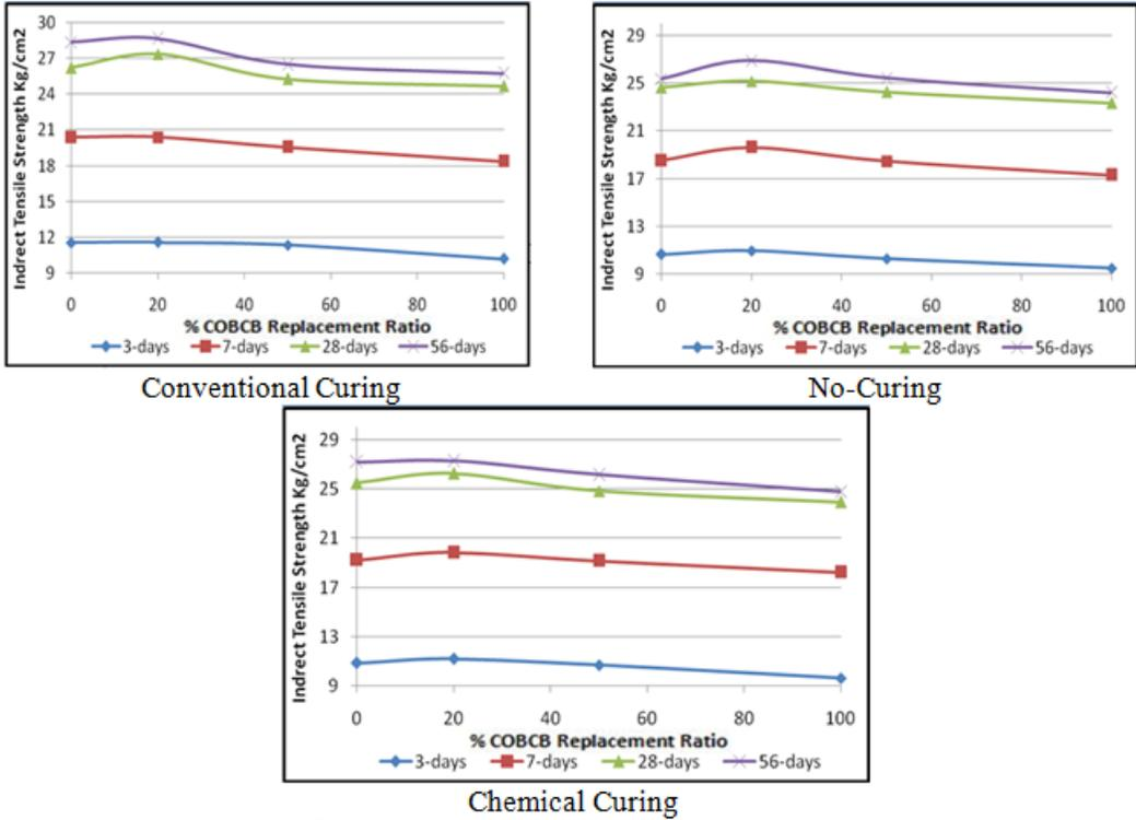
Fig. 5. Effect of % (COBCB) on indirect tensile strength.
