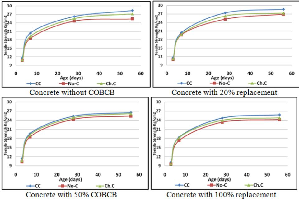
Fig. 8. Effect of curing type on indirect tensile strength.
