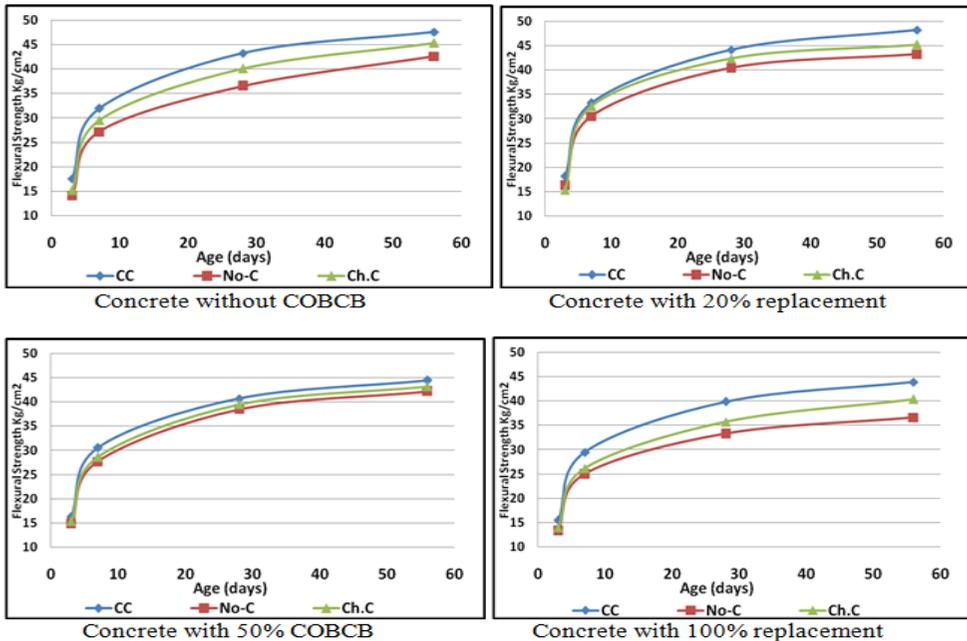
Fig. 9. Effect of curing type on flexural strength.
