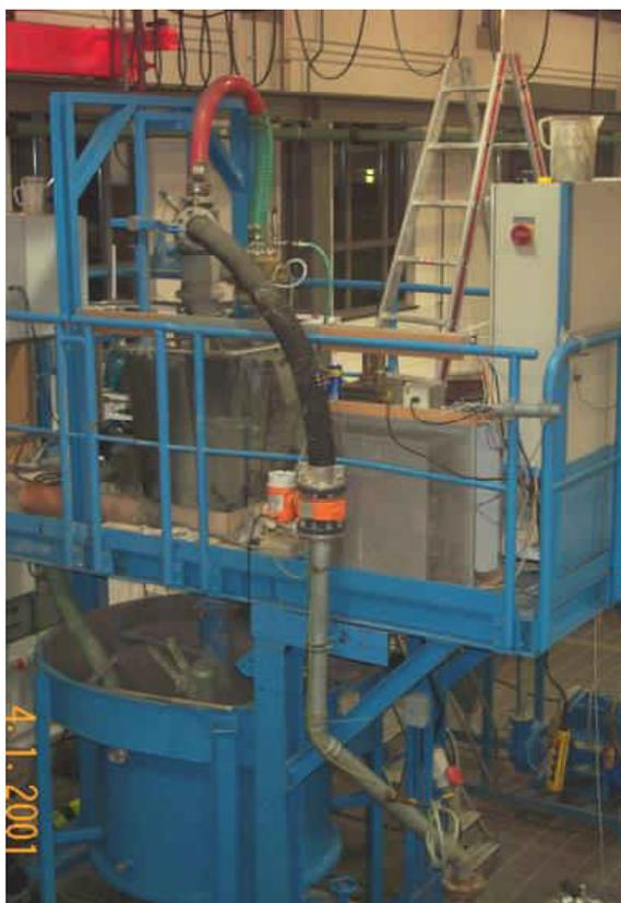
Fig. 1b: Photo of semi-technical controlled hydrocyclone plant
