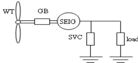
Fig.(1): Schematic representation of the wind energy system
