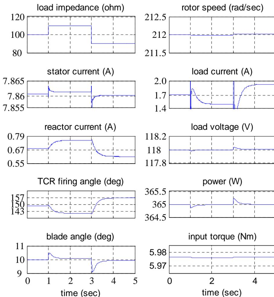
Fig. (7) Simulation results of the proposed scheme with step change in load impedance with parameters variations.
