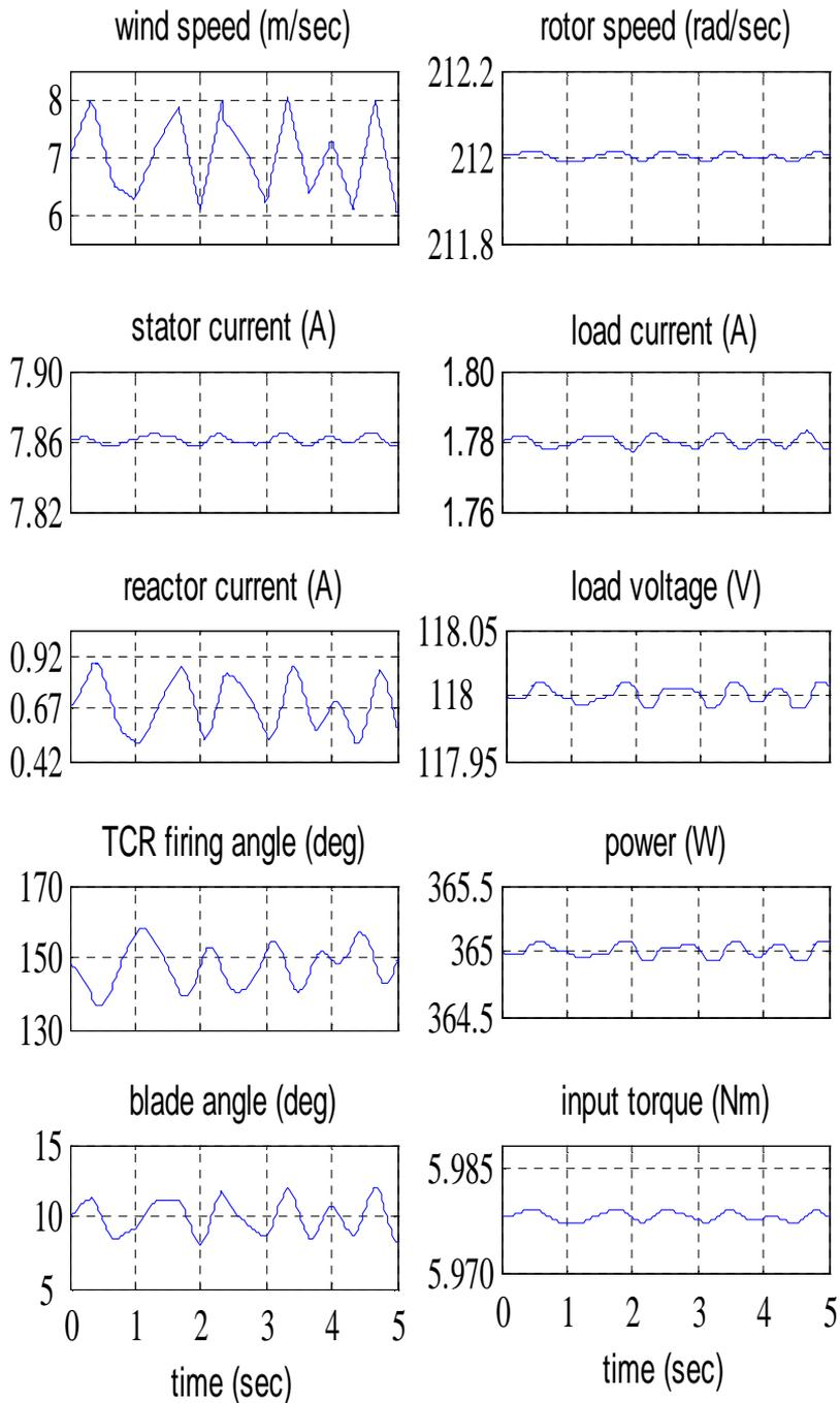
Fig. (6) Simulation results of the proposed scheme with step change in wind speed with parameters variations.
