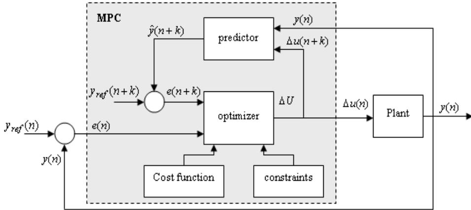
Fig. (2): Basic structure of model predictive control
