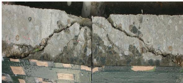
Fig. 13 Punching shear failure
