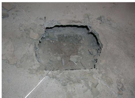
Fig. 15 Typical discontinuity on the top surface of the slabs after failure
