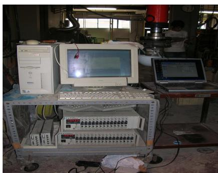
Fig. 2 Adrec recording system
