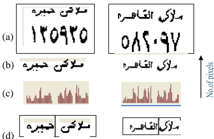
Fig.11. Vertical projection for the registration row
