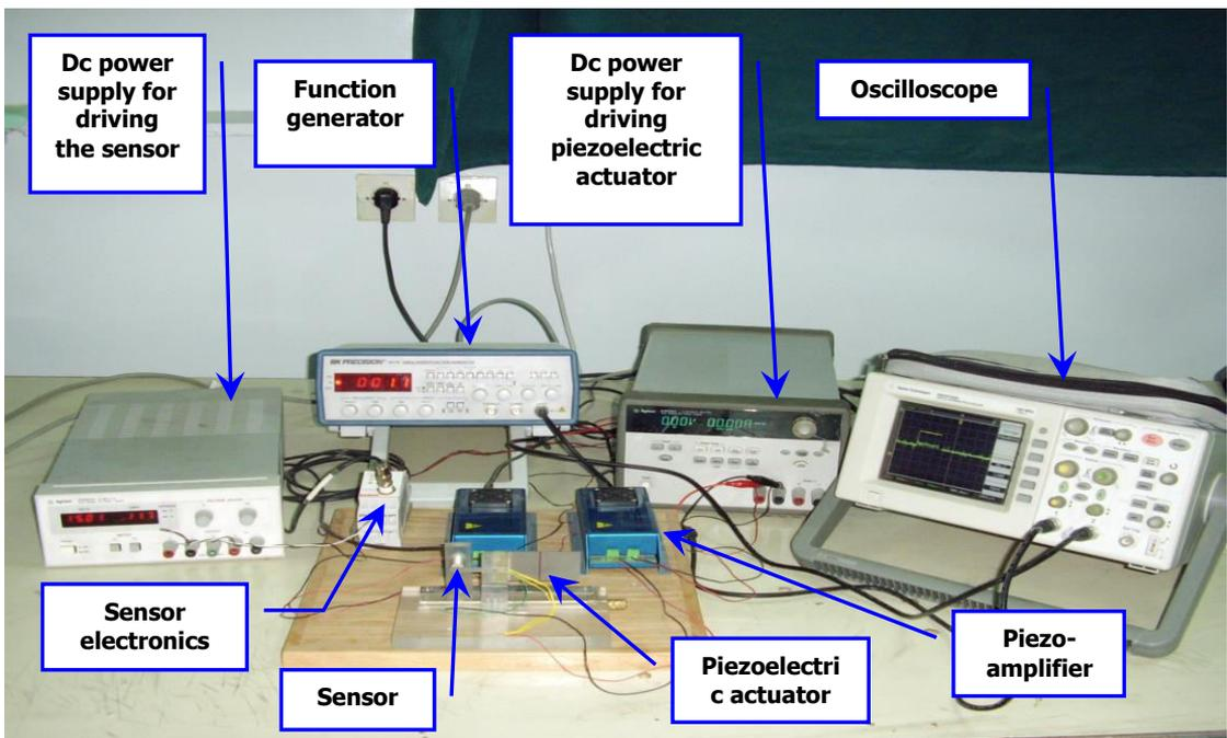
Figure (3) Photographic view of the experimental setup
