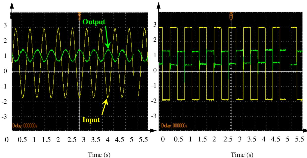
Figure (8) (a) Sine wave signal  $v = 3 \text{ V}, f = 1\text{Hz}$  (b) Square wave signal  $v = 3 \text{ V}, f = 1\text{Hz}$
