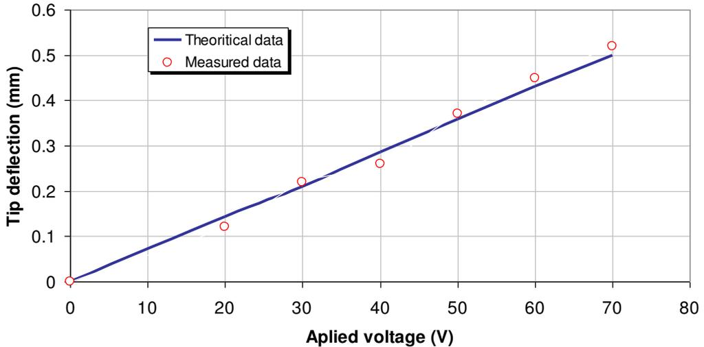
Figure (6) The static deflection of a bimorph actuator at  $x=L$  versus the applied voltage
