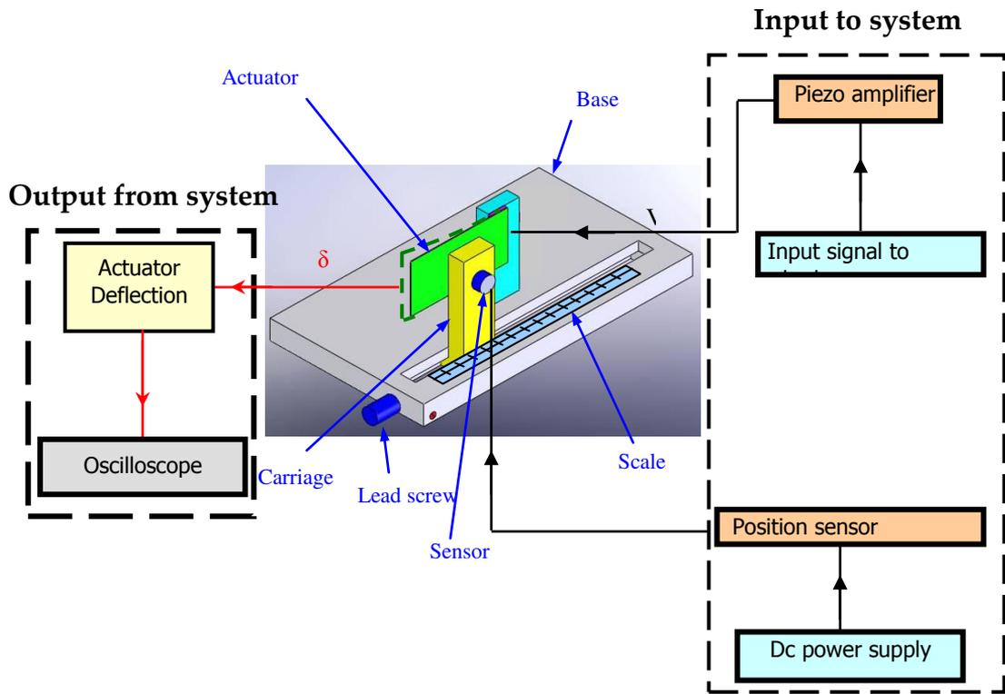
Figure (4) General layout of the experimental setup
