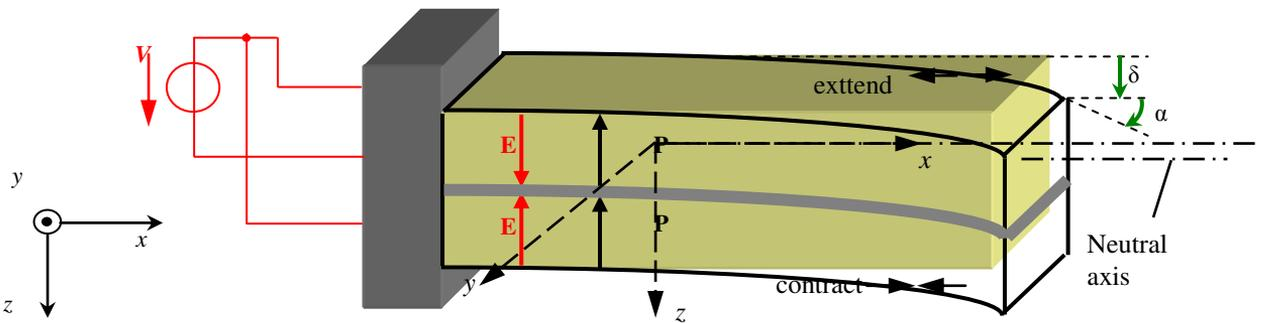
Figure (2) Basic intensive parameters of Bimorph actuators after applying electric field
