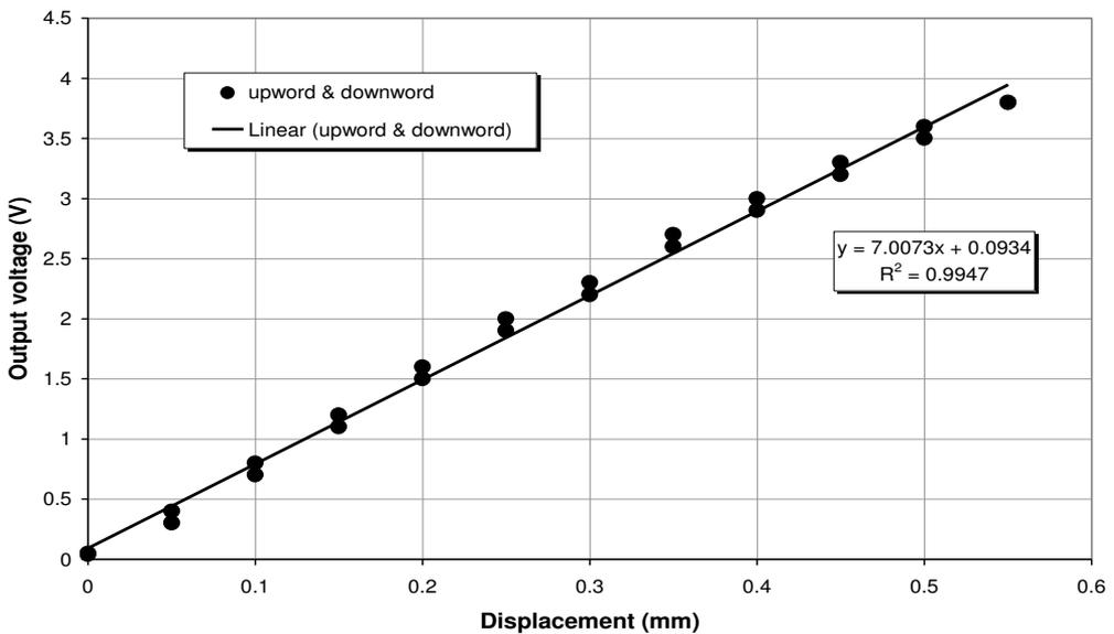
Figure (5) Calibration curve of the position sensor
