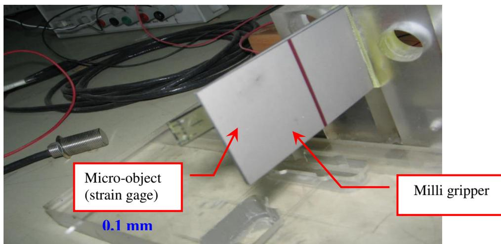
Figure (10) The micromanipulator carries a small object (strain gage)
