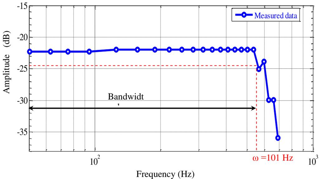
Figure (9) Variation of the deflection with the frequency for bimorph actuator
