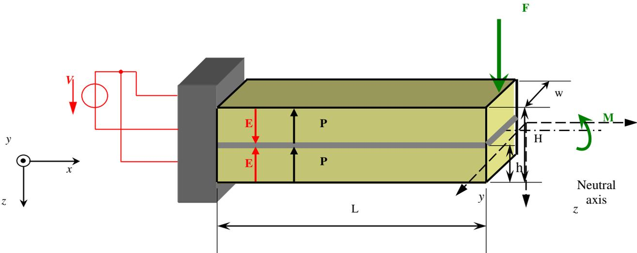
Figure (1) Basic dimensions, extensive parameters, polarization, and applied electric field acting on the Bimorph actuator
